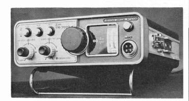
Following the worldwide success of the TS700, Trio have taken the TS700 basic design and packaged it for 2 metre SSB mobile use. The TR7010 sets new standards in receiver sensitivity and low spurious emission on transmit. Operating CW and SSB from 144-1-144-3 MHz, the TR7010 covers all CW, SSB and beacon activity. 40 5 kHz channels plus VXO and RIT provide continuous coverage, 8 extra channels can be used, without returning, in the range 144-145 MHz by fitting auxiliary crystals.
