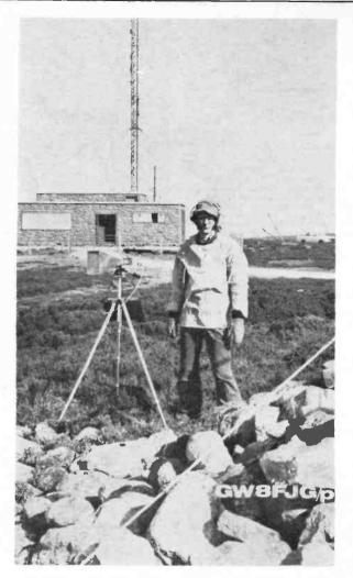
The three-centimetre rig operated by GW8FGP/P, running 10 mW with a Gunn oscillator and using a horn antenna giving about 22 dB of gain. See notes on p.397, September issue, and the narrative.
