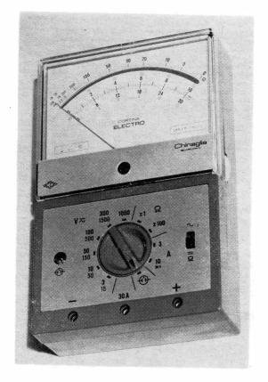
The Chinaglia Electro is a new 19-range multi-meter designed for electricians' use and general hard work. The voltage-current ranges go up to 1000v. DC/1500v. AC and 30 amps., resistances from 10K to 1M, with a continuity-check facility. Internal 1½v. batteries energise the resistance ranges.
