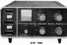
KW 1000 Linear Amplifier. 10-80 metres. 1200 watts PEP input max. Designed to be input max. Designed to be "driven" by KW 2000A/B/E or other Unit of similar power rating. In-built 2.5 Kv. PSU. PA tubes pair T160L. Very quiet in operation.
