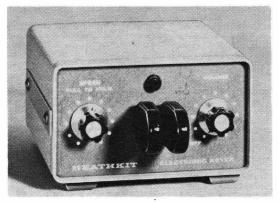
(Upper) The Heathkit HD-1416 Code Practice oscillator, which operates from a 9v. supply, and comes complete with key and phone jack, in a home-constructor kit costing 27.000. (Below) The Heathkit HD-1410 electronic keyer, with adjustable dotdash paddles for speeds from 10 to 35 w.p.m. It can be AC or DC powered and costs £29.70 in kit form.
