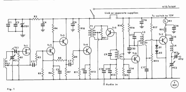
Fig. 1. Circuit of the Sideband Tx for Top Band
