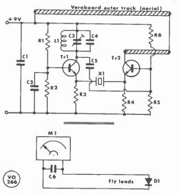
Values for the Test Oscillator/RF Sniffer can be: C1, C2, .001  $\mu$ F; C3, 10  $\mu$  $\mu$ F trimmer; C4, 10  $\mu$  $\mu$ F silver mica; C5, 47  $\mu$  $\mu$ F s/m; C6, 220  $\mu$  $\mu$ F, disc; R1, R6, 15K; R2, R5, 2.2K; R3, R4, 100 ohms; Tr1, Tr2, BC107; Coil, 5 turns 20g, to  $\frac{1}{2}$ -in. dia. And for the Sniffer, D1 is 1N4148 or similar; M1, 0-500  $\mu$ A meter; and X1, 14 MHz crystal (see lext).
