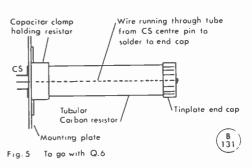
Fig. 5. Coaxial dummy load, constructed as shown, will be useful even up to VHF. The mounting-plate can be one face, or a sealed container on which the lid fits tightly. Filling this with oil of ordinary engine grade will greatly improve the wattage rating, while the container itself will function as an RF
