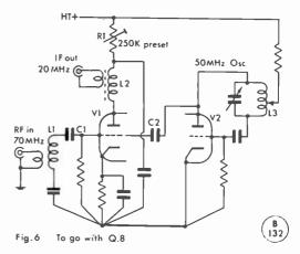
Fig. 6. This arrangement could allow the local oscillator to "see" the Ae. terminal, so that in practice an RF stage would be used. L1 is tuned to mid-band. C1, 33  $\mu\mu$ F, and C2, 10  $\mu\mu$ F, are the important values. Effectively, R1 adjusts the anode potential of the mixer, V1, to give best noise performance at the available oscillator output. The valve could be a 12AT7, or similar double-triode.
