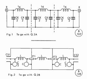
Fig. 2. The low-pass filter is built into a long narrow box (with a tight-fitting lid, not shown) divided into three sections by internal screens. These screens are pierced by feedthrough insulators, Ft, and the ends of the box carry coaxial sockets, CS. Coils are arranged as shown and capacitors connected by short leads to an adjacent earth tag.
