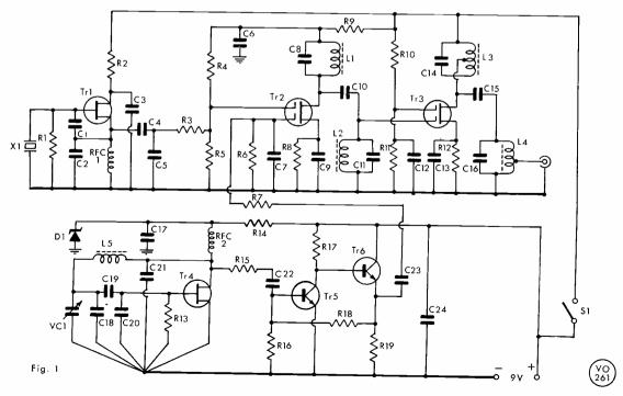
Fig. 1. Circuit of the VFO
