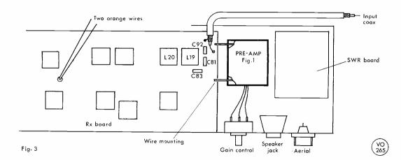
Fig. 3. The Preamplifier incorporated into the Liner-2. For some further details see text. The gain control enables input level to be reduced in the presence of strong signals.
