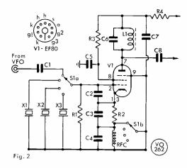
Fig. 2. Transmitter CO modified for VFO input
