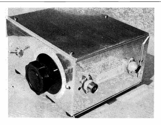
Converter as completed, with coax input-output sockets
