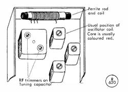
Interior layout of typical Japanese-type MW Rx
