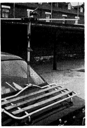
Neat mounting for a J-Beam two-metre crossed dipole array, shown by G8ERX/M at the Humberside Rally. It is fitted to the luggage rack of his Ford Escort and the whole assembly can be dismounted without leaving any scars.
