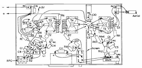
Fig. 2 UNDER CHASSIS LAYOUT AND WIRING
