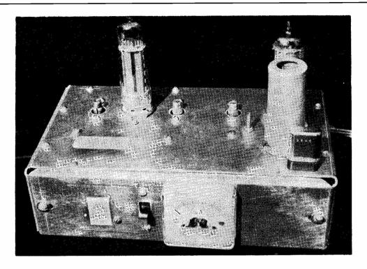
General appearance of the Four-Metre RF Unit. Meter is switched to read grid or anode current.
