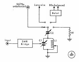
Basic values for this ATU can be, for all-band coverage: C1, 300-0-300  $\mu_{\rm B}{\rm F}$  split stator; C2, 425  $\mu_{\rm B}{\rm F}$ ; R1 for dummy load, carbon types to make up to 50 ohms and dissipate the power required, in this case 10 watts, so that two 5-watt 100-ohm resistors would do. For coil details see text.
