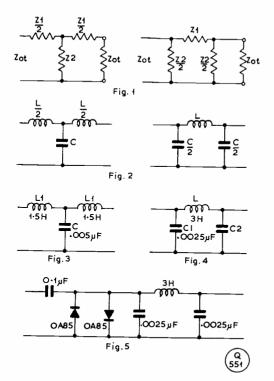
constant-k and as Z1.Z2 = R<sup>2</sup>, therefore R =  $\sqrt{L/C}$ . And without proof the cut-off frequency *fc* is given by  $fc = I/\pi\sqrt{LC}$ .
