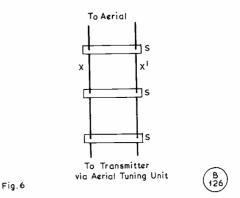
Fig. 6. To answer Q.10(A). Open-wire balanced feeder-see
