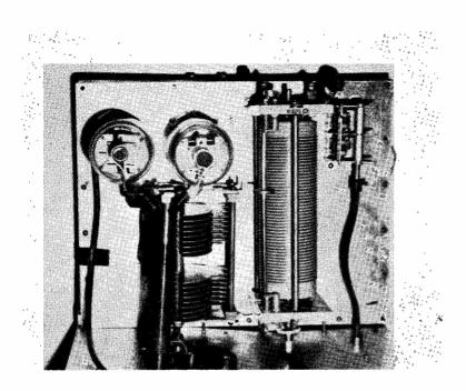
Layout of the double-813 Linear Amplifier described by GW4BCD in the last issue—it can run a cool 600 watts.
