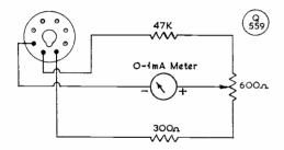
Circuit of the Plug-In S-Meter
