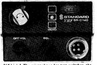
24" high 1 The microphone has two switches, the normal PTT switch plus the MEMO switch. A flick of the switch and the transceiver overrides the Channel selector and you can transmit or receive on another frequency. The C140 takes the CVI10 Remote VFO or SY-200 Synthesizer and comes complete with microphone, line filter and mounting hardware.
