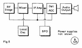
Fig. 5. To answer Q.7. Block diagram of a superhet receiver of conventional design.
