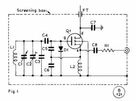
Fig. 1. To answer Q.2(B). Seiler Oscillator using 1GFET. It would be used with a buffer stage (see text) and values could be : C1, 100 pF; C2, 25 pF, trimmer; C3, 100 pF, silver mica; C4, 330 pF, silver mica; C5, C6, 630 pF, silver mica; C7, 0.1  $\mu$ F; C8, 0.022  $\mu$ F; R1, adjust for optimum with buffer stage connected; L1, 17 turns 20g., 1-in. dia. by 1-in. long; L2, 2.5 mH RF choke; D1, 1N914; Transistor, 1GFET or 3N128; FT indicates feed-through capacitors.
