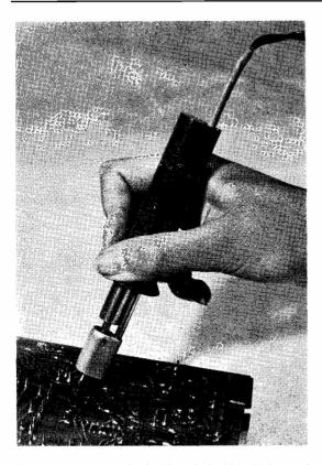
The one-hand-operated Picard soldering/desoldering tool is an ingenious device which can be operated either to "undo" soldering (the molten fluid being removed by suction) or to make soldered joints in the usual way. Weighing only 50 grammes it is rated at 20 watts and runs off an 8-volt supply. Price is  $\pounds 6.49$ , with stand.
