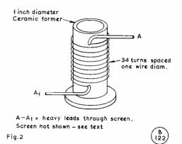
Fig. 2. To answer Q.3(A). Tuning coil for 1.8 MHz VFO.
