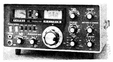
This is a new and improved version of the well-known FTI01. It is fitted with a cooling fan as standard and is improved in several respects:-
