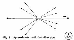
Fig. 5. Presumed radiation directivity on the HF bands—see text.
