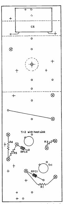
Tri and Tr2 mounted this side (laminate) with leads pushed through
