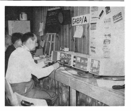
worked using KW-2000 and FT-401 transceivers, into large antennae. Their most interesting QSO was with II4FGM, Bologna, at Marconi's birth-place.
