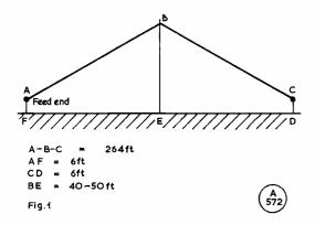
Fig. 1. General layout of the G3LCK aerial system.
