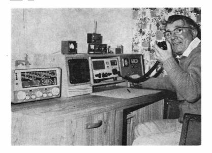
E. Waddington, G8EDI, 18 Barnwood Road, Earby, Colne, Lancs. has an HW-17 with FET pre-amp., all built into a neat console, with outside an 8-ele flat-top at 35ft. The Rx on the left is a Mohican GC-1U, the Heathkit full-coverage transistor receiver.
