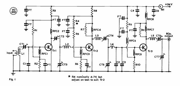
Fig. 1. Circuit of the two-metre Transistor PA.
