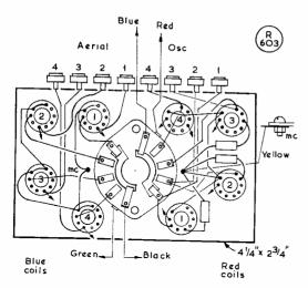
Fig. 3. Wiring of the Coil pack
