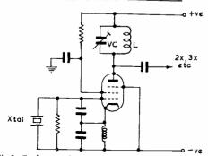
Fig.8 Typical oscillator with harmonic output
