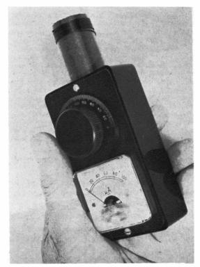
An indicating absorption wavemeter, using a plastic box as container to minimise hand-capacity effects, and an 0-100 microamp. m/c meter as the resonance indicator.
