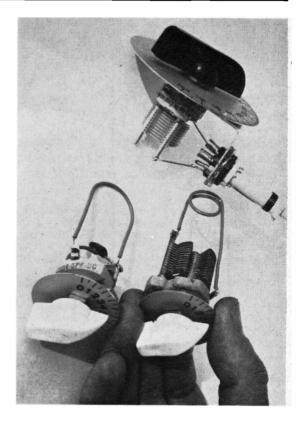
Single range absorption wavemeters of the type discussed in the text for 138-148 MHz and 42-160 MHz, also (at top) a five-range wavemeter with plug-in coils for 1.8 to 150 MHz.
