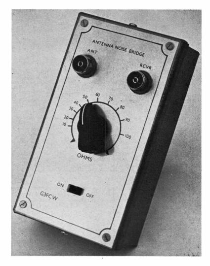
The completed Ae. Noise Bridge as described in the text by G3FCW. The coax sockets and switch can be fitted using countersunk bolts which are hidden when the front panel is in place.
