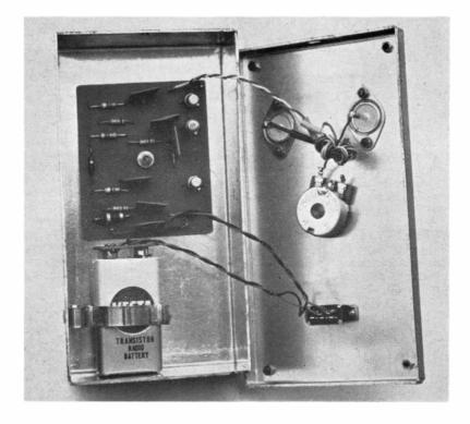
Interior lay-out of the Noise Bridge as built from the "Cambridge" kit —see text. The toroid is suspended in the wiring between the coax sockets and the reference potentiometer.
