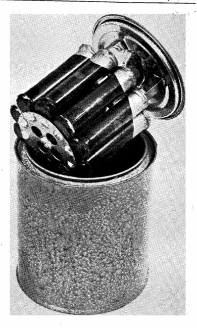
This detail is to show the holes in the bottom disc to help circulation of the oil coolant—which, in this simple application, can be ordinary domestic cooking oil.
