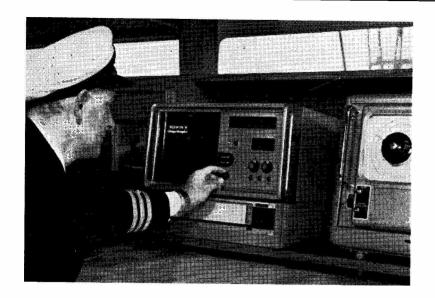
The new Redifon "Omega Navigator" receiver will give a ship positions accurate to within about one mile on ocean passages across the world. It is, of course, a satellitereferred device and is now installed in the new ship m.v. "Orbita" of the Pacific Steam Navigation Co., Ltd.
