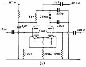
Fig. 2. At (A) the circuit of a typical transistor product detector and (B) a similar valved detector.
