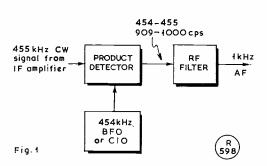
Fig. 1. Block diagram to show how an audio signal is derived from a product detector.
