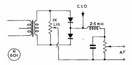
Fig. 4. Circuit diagram of a balanced product detector for optimum AM rejection—see text.
