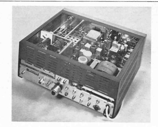
Half-rear view of the FT-DX560, showing rear chassis-drop connecting points.
