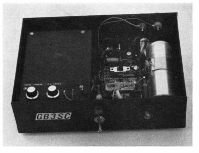
The new GB3SC keyer unit for the Sutton Coldfield 70-centimetre beacon. It was designed and constructed by Brian Coleman, G8AZU, as a free donation. Intended for continuous operation, it is all-solid-state using IC's and the quality of the keying has been commented upon most favourably.
