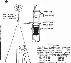
Telomasts telescope down to 10', are rotatable and are ideal for fixed station installations, field days and
