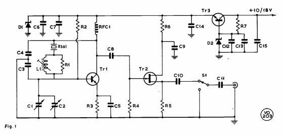
Fig. 1. Circuit of the VXO by G8FVN — see text.
