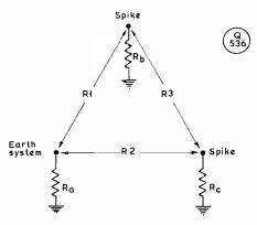
Method of measuring the resistance of an earth system E, using temporary earth spikes set out in a triangle. The resistances R1, R2 and R3 between pairs of points are measured; the resistance of E can then be calculated as described in the text. Other uses of the tests and the simple formulae derived are also explained.
