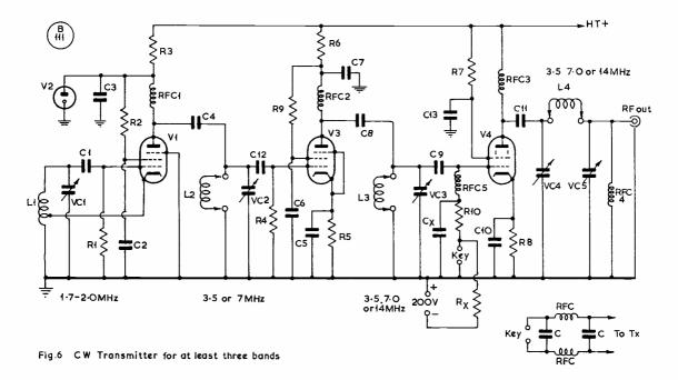
Fig. 6. (To answer Q.8). The items involved in the chosen keying system should be clearly noted, as the answer requires a careful and thorough explanation of the working of your method. Plug-in colls save time; but it becomes necessary to indicate on the drawing the frequencies to which the various circuits can be tuned.
