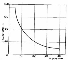
Fig. 1 Max. Load Current Input Output Voltage Differential
