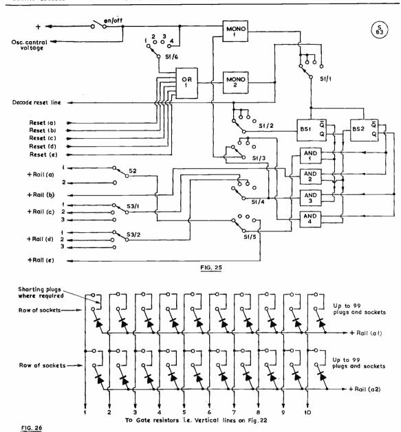
Fig. 25. Block diagram for M/S data generator. Fig. 26. Plug-socket arrangement for build-up of callsigns.
