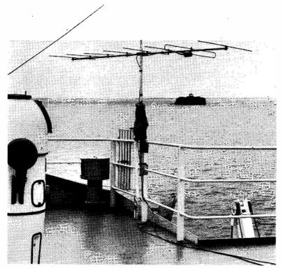
The 8-ele Yagi used by G3UGF/MM in his operations from the m.v.
