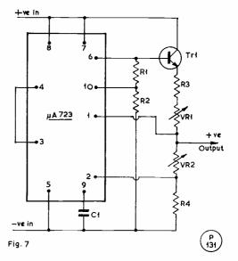
Fig. 7. HV regulator with current limiting and external pass transistor. The values are: C1, 100 pF; R1, 1.2K; R2, 8.2K; R3, three-ohm 5w. wire-wound; R4, 6.8K; VR1, 100-ohm 25w. w/wound; VR2, 20K linear potentiometer; and Tr1, 2N3055. (All fixed resistors rated  $\frac{1}{2}w.$  high-stab., except R3.)
