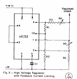
Fig. 5. HV regulator with fold-back current limiting, for which values are: Cl., 100 pF; R1, 1.2K; R2, 8.2K; R3, 50 ohms, 5w. wire-wound; R4, 100 ohms, 10w. w/wound; R5, 20K linear potentiometer; R6, 6.8K. All fixed resistors rated half-watt, high stability, except as indicated.
