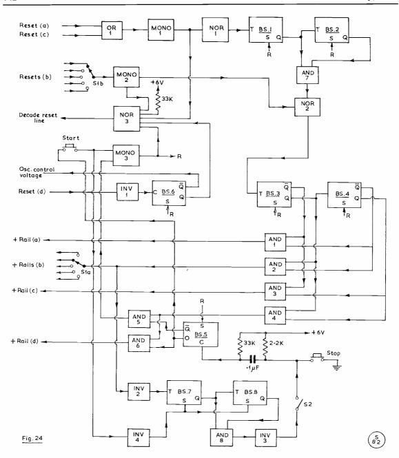
Fig. 24. Block diagram of complete CQ generator.
