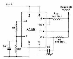
Fig. 3 a. Basic Low Voltage Regulator +2 to 6 volts
