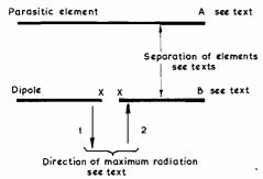
Fig.7 b. Directional aerial for Transmitting on an HF Band
