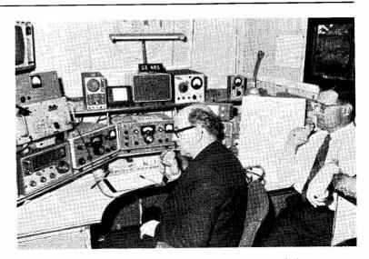
Station of G3NRS, well-known member of the Scarborough Amateur Radio Society. He runs a very nice all-band layout, fitted into a console for tidiness and convenient operation. This is the sort of installation which is quite easy to fabricate, using hardboard, lin. batten and a bit of imagination.
