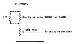
Modifications to Line oscillator for 625 line operation
