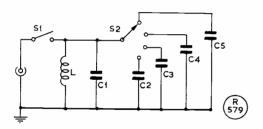
Fig. 3. Audio selectivity unit for JR-310, for which values can be : C1, C3, .047  $\mu$ F, 200v.; C2, .02  $\mu$ F, 200v.; C4, 0.1  $\mu$ F, 200v.; C5, 0.3  $\mu$ F, 200v.; and L, 120 mH.
