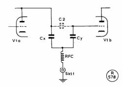
Fig. 2. Modification of AF sub-assembly in the JR-310 for provision of the external audio selectivity unit. Values are: Cx, Cy, .01  $\mu$ F, .400v.; RFC, 1.5 mH; Sk1, screen jack socket. Note that C2 is removed from the circuit board.
