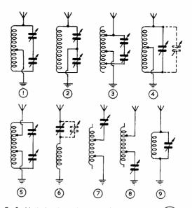
Fig.3 Methods of coupling Long wire and other End-fed aerials
