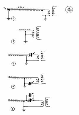
Fig.2 Circuits at the Link or Input side of Coupler
