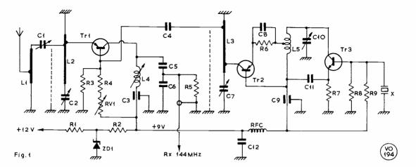
Fig. 1. Circuit of the 70-Centimetre Converter.
