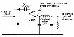
C1 inserted to prevent positive bias being applied to video amplifier arid
