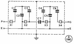
Fig. 4. Circuitry of a 3.7 kHz filter for the 455 kHz IF of the Trio JR-310. C1, C3, C4, C6, 270  $\mu\mu$ F; C2, C5, .001  $\mu$ F; C7, 39  $\mu\mu$ F; X1, X2, X3, X4, Clevite identical resonators, Type TF04-442; all capacitors should be good quality silver-mica or polystyrene-foil.
