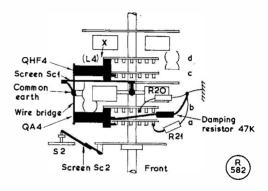
Fig. 6. General impression of the JR-310 coil pack showing, in heavy line, the position of additional components for the Top Band modification.
