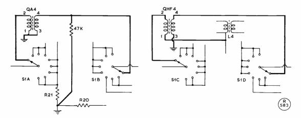
Fig. 7. Partial circuit of the JR-310 coil pack, with the Top Band modification in heavy line.
