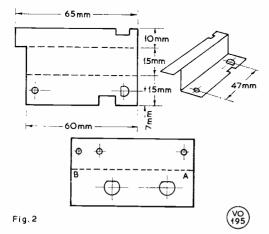
Fig. 2. Above, drilling diagram for the copper-clad board. Centre, showing the folding and drilling for the screen between L1 and L2, using 22g. copper sheet. Below, mounting bracket for the BNC connectors.
