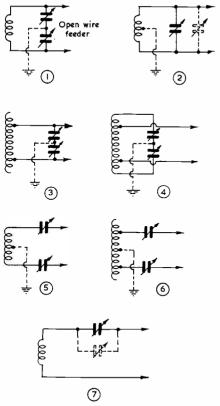
Fig. 4 Circuits for Zepp, Doublet or Double Zepp,
