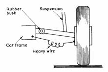
Fig.3 Grounding Front Suspension
