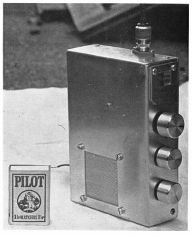
General appearance of the completed two-metre personal portable, as designed and constructed by G3TDZ, with a size comparison. The speaker is behind the grille. The Tx runs two watts and more than 100 stations have been worked using simple antennae.
