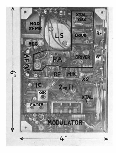
Showing general layout inside the chassis with main sections of the circuit identified—compare with circuit diagram The size of 6in, by 4in. would be quite comfortable for hand-held operation.
