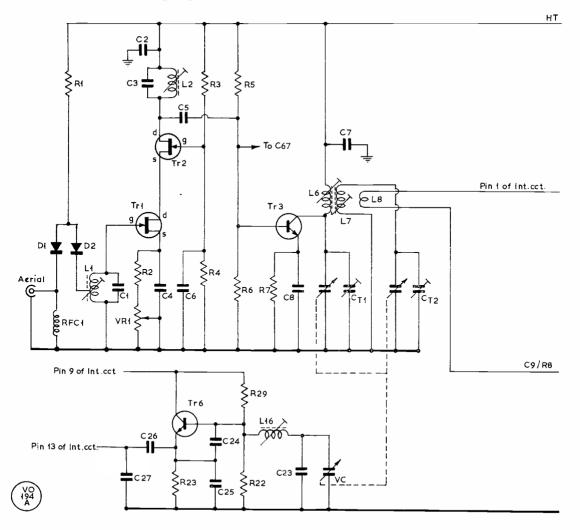
good, obviously the S2K19's could be replaced by 2N3819's or UC734's, etc. For those wishing to be more "with it", one of the new dual-gate Mosfets such as 40673 or 40820 should make a lively RF stage.
