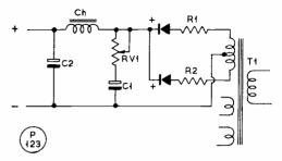
will allow the voltage to be reduced with any capacitor input circuit. The method is most suitable for equipment imposing a steady HT load.
