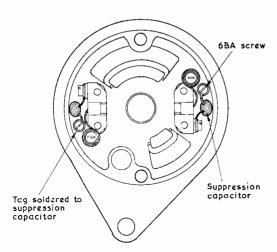
Fig.1 Dynamo End Plate
