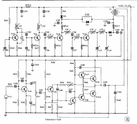
The G3TDZ Two-Watt Transmitter Circuit.
