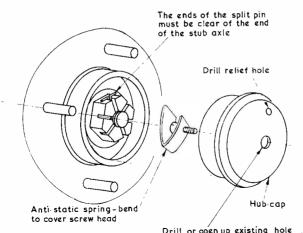
Drill or open up existing hole to clear 4BA screw (No. 25 drill) The hole must be in exact centre of cap
