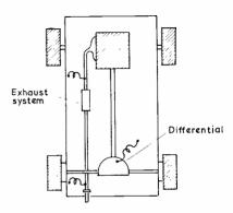
Fig. 5 Additional grounding points
