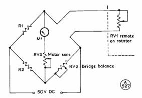
Circuit of the beam direction indicator described by G8CHP, for mounting at the operating position. Values are: R1, R2, 10K; RV2, 470 obms; RV3, 5K; meter 0-1 mA. RV1 is a 470-ohm potentiometer activated by the rotator, mounted in some convenient manner to obtain drive—see text.
