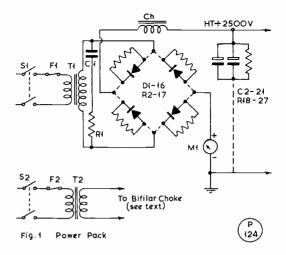
Fig. 1. Suitable PSU for the 813 Linear discussed in the text. C1, 500  $\,\mu\mu\mathrm{F}$ , 3 kV.; C2-C21, 60 + 250  $\,\mu\mathrm{F}$ , electrolytic, 350v. working, ten in series-parallel; R1, 1.5K, 5w.; R2-R17, 470K, ½w., 4 in series across each diode; R18-R27, 470K, ten in series; Ch., 5-25 Hy, rated 250 mA+; D1-D16, see text; T1, 1000-0-1000v. at 250 mA; T2, 10v. at 10 amps for 813 heaters.
