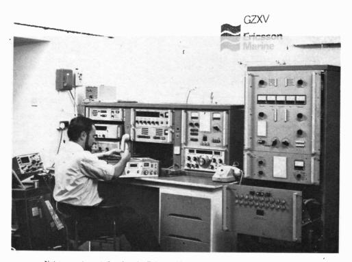
Not an amateur station, but the Ericsson Marine commercial demonstration set-up, allocated the ship callsign GZXV, and established at the Norway Trade Centre, Pall Mail, London, to provide advance training for ships' radio officers in the servicing and maintenance of Ericsson equipment. In charge is Bryn Tinton, G3SWC, who has himself served at sea with Cunard, in their ships ''Atlantic Causeway'' and ''Atlantic Conveyor'', fitted with the most sophisticated marine radio equipment.
