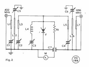
Fig. 2. The tripler circuit for 432-1296 MHz, where line dimensions and mechanical layout become critical.
