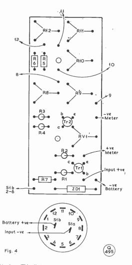
Fig. 4. This diagram represents the wiring layout if the board shown in Fig. 3 is used. Dimensions are such as to fit into a box or cabinet 4in. wide by 3in. deep.
