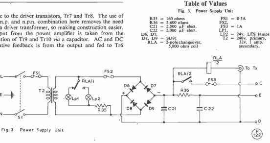
Fig. 3. Suitable Power Supply Unit.
