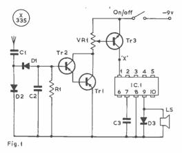
Fig. 1. The main unit, for which values can be : C1, C2, .001  $\mu$ F, mica ; C3, 0.33  $\mu$ F, paper ; R1, one megohm ; VR1, 50K, carbon ; D1, D2, D3, BAX13 or similar ; Tr1, Tr2, 2N4288 ; Tr3, BYF51 ; IC1 (integrated circuit) used, see text ; LS, any small transistor radio speaker.
