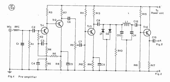
Fig. 1. Circuit of the Preamplifier.
