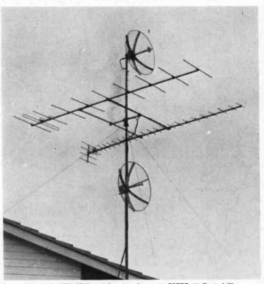
(Above) the VHF/UHF aerial system in use at G3ZEZ, 16 Kestrel Way, Clacton-on-Sea, Essex. At top is a 3 ft. dish for 23 centimetres—then a 10-ele Yagi for two metres—below it a 24-ele array for Seventycems and lastly a 3ft. dish for 3 centimetres. Mounted on a rotatable mast, the whole of this assembly is home-built. At lower left is the station of G3ZEZ, all the VHF gear having been constructed by him. Altogether, a very workmanilke job, on which he is to be congratulated.
