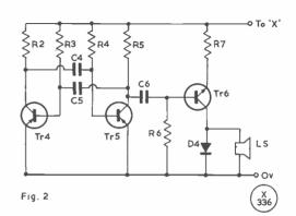
Fig. 2. An alternative power oscillator arrangement. In this, C4, C5, are .0022 µF; C6 is 0.1 µF; R2, R5, 4,700 ohms; R3, R4, 680K; R6, 1000 ohms; R7, 22K; D4, BAX13 or the same; Tr4, Tr5, 2N4288; Tr6, BYF51.
