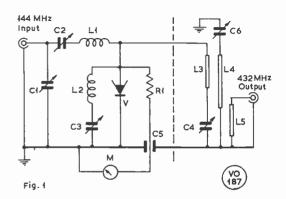
Fig. 1 Circuit of the 144-432 MHz varactor tripler, discussed in the text.
