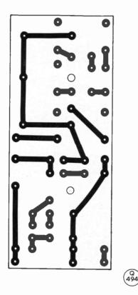
Fig. 3. While any tidy method of construction can be used, a professional-looking job will result with a printed circuit board. Etching and drilling details for a suitable layout are shown here.
