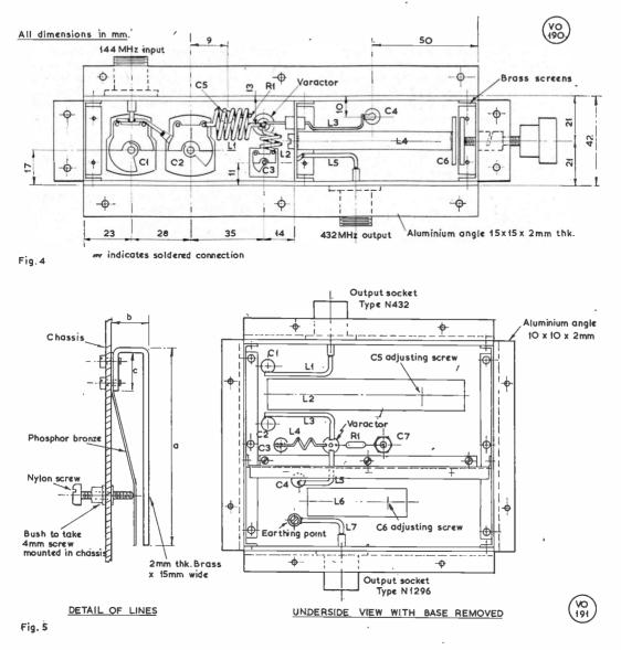
Fig. 3, Fig. 4 and Fig. 5 show general constructional procedures. all dimensions shown being in millimetres.
