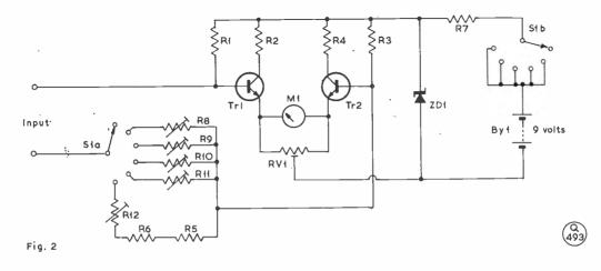
Fig. 2. Circuit of the high-impedance voltmeter complete as discussed in the text.
