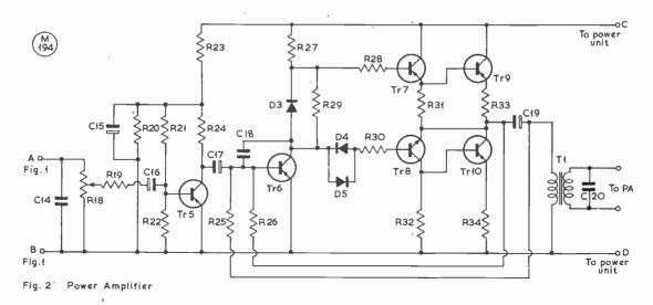
Fig. 2. The Power Amplifier section.
