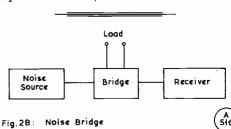
The Omega-T unit has a measuring range from zero to 100 ohms, which is less than that of the Antennascope. As it stands, the range is adequate for use with 50 and 70 ohm coaxial and balanced feedlines. Later in this article, it will be shown how a quarter-wave line can be used in conjunction with the bridge to extend the measuring range to much higher impedances.
