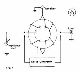
Fig. 4. Combined quadrafilar-wound coupling and balun bridge, as used in the Omega-T circuitry—see text.
