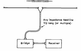
Fig.7B Remote measurement of balanced derial
