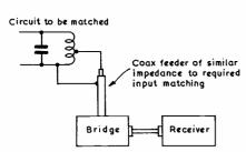
Fig. 10. Adjustment of receiver input circuits.
