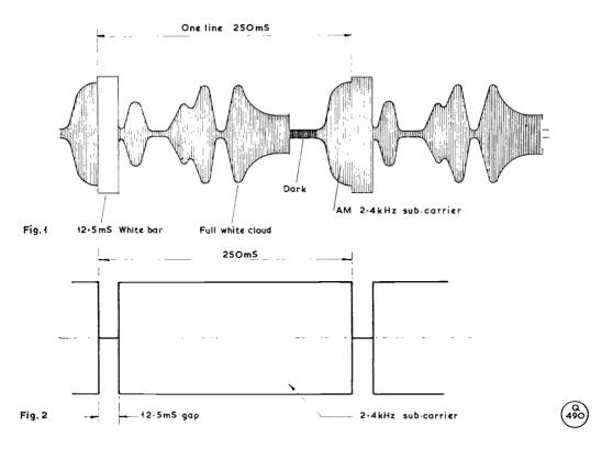
Fig. 1. Typical line from a picture sent by an APT weather satellite—see text. The full white edge of the picture lasts 12.5 mS, the remainder of the 250 mS being cloud-cover information. Fig. 2. The phasing signal which precedes the sending of a picture. This is for the purpose of getting the 4-cycle line time-base in step with the picture transmission.
