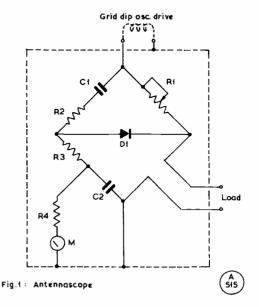
Fig. 1. Circuit of the Antennascope. Values are: C1, C2, 500  $\mu\mu$ F or near but matched to within 1%; R1, 100-ohm noninductive potentiometer, carbon type, w/wound not suitable; R2, R3, 100-ohm non-inductive carbon, matched to within 1%, actual value not critical; R4, IK  $\frac{1}{2}$ -watt carbon; D1, OA81 or similar diode; Meter, 0-200 microamp.
