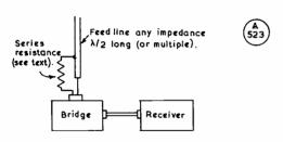
Fig. 9 Measurement of very low impedances
