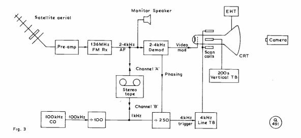
Fig. 3. Block diagram to show the layout of units for reception of Weather Satellite pictures.
