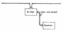
Fig.7A. Direct measurement at feed point of gerial
