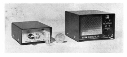
times must be all but equal, which is not uncommon with this type of relay. Contacts are rated reasonably, although they could hardly be expected to drive a cathode-keyed 813—they certainly cope quite happily with anything in the way of normal voltages and currents; and both the Monitor and the Keyer itself are of equal capability, implying that if the two units are coupled, one of the contacts can be used for driving the transmitter, and the other for, say, muting the receiver.
