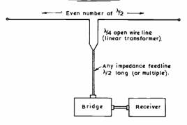
Fig. 8B Measurement of long-wire aerial at voltage point
