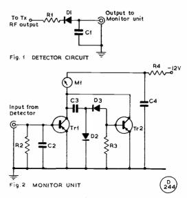
Fig. 1. The detector circuit, in which C1 is .01  $\mu$ F disc ceramic; R1, 68K; and D1, OA81. In Fig. 2, the monitor unit, C2 is .001  $\mu$ F, disc ceramic; C3, 0.22  $\mu$ F; C4, 0.1  $\mu$ F; R2, 27K; R3, 68K; R4, 12K; D2, D3, OA81; Tr1, Tr2, OC45; and M1, 0-1 mA m/c meter.
