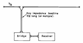
Fig. 8A. Measurement of long-wire aerial at current point
