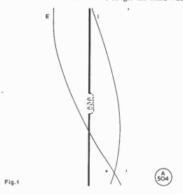
Fig. 1. Voltage (E) and current (I) distribution on a one-third  $\mathbf{w}/\mathbf{l}$  centre-loaded aerial. For the whip construction discussed in the article, the total length for Top Band is less than 10ft.
