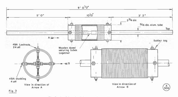
Fig. 3. Careful study of these drawings will make the constructional details clear. A Top Band radiator of this kind can be used effectively either /P or /M and also as an indoor system for 160 metres.
