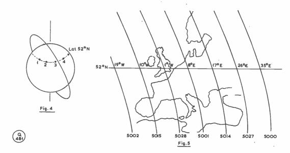
Fig. 4. The plane of the satellite remains fixed in space, while a point on the surface of the rotating Earth will move successively through the positions indicated in the time the satellite takes to make one orbit. Fig. 5. Outline map of Europe showing the satellite tracks given in Table I, opposite.
