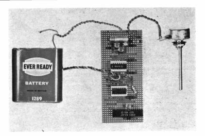
The Keyer unit complete, as designed and constructed by G3KPT. The potentiometer is for speed control. Assembly is on a piece of 0.1in. "Veroboard".
