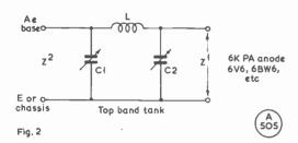
Fig. 2. The \(\frac{1}{2}\)rd.-wave aerial can be fed by direct connection to the conventional pi-tank circuit for Top Band, for which L, C1, C2 here have usual values.
