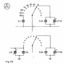
Fig. 2B. The preselector modifications for Top Band in the Drake 2-B. CIA, C2A, are .001  $\mu F$  silver mica. CTIA, CT2A, 700  $\mu \mu F$  compression-type trimmers—see text.
