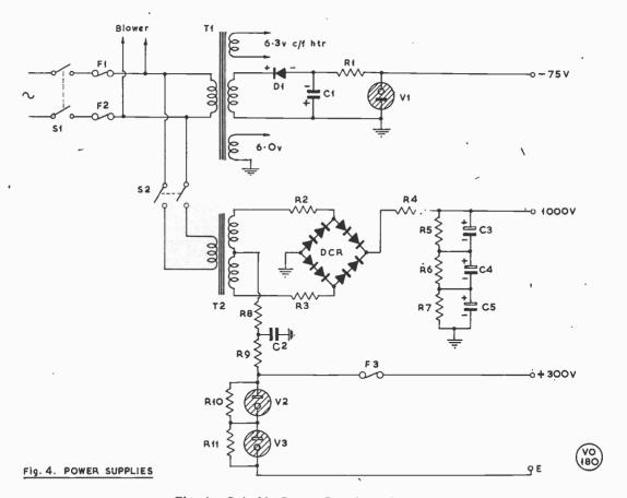
Fig. 4. Suitable Power Supply Unit for the 70-Centimetre Tripler.
