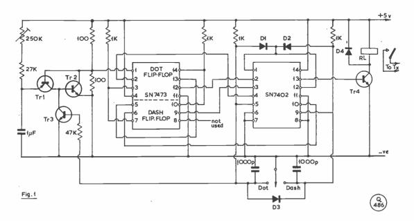
Fig. 1. In this circuit, Tr1 can be BCY-70 or BCY-71; Tr2, Tr3, Tr4 are BC-107; D1, D2, D3 could be OA91; D4, BAX-16 or any silicon diode; and RL is a 6v. reed relay—see text. The integrated circuit units are SN7473N, or similar.
