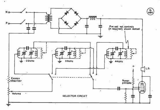
Receiver unit for "Wired Wireless," as used pre-1939.
