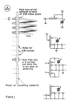
Fig. 1. Coil construction details and possible circuit variations for the ATU described in the article. The coil must be mounted on a panel of good insulating material.
