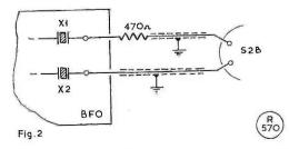
Fig. 2. As explained in the article by G3DNF, an anti-parasitic resistor is desirable to eliminate "birdies" that may be produced by the BFO in some production models. This is how it can be fitted. The image rejection of this receiver is good, and cross modulation is not noticeable under normal operating conditions. However, the RF gain and tuning need careful adjustment for the best results to be obtained on 7 MHz. This is nowadays usual with most modern receivers.
