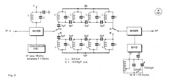
Fig. 2. Essential circuitry to reproduce narrow filters for CW reception—see text. The BFO coil can be Mullard LA80, of 265 turns of 34g, with the cathode tap at the 241st turn.
