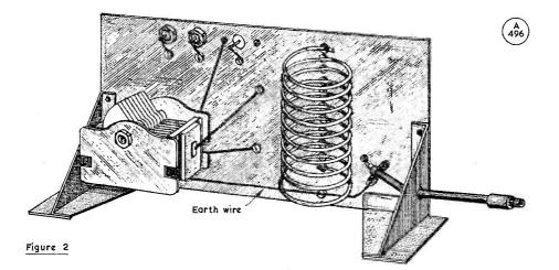
Fig. 2. General layout of the ATU, on its insulated panel. For outdoor operation, the unit should be enclosed in a protecting cover.
