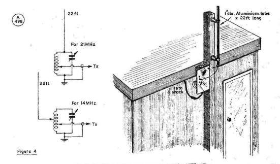
Fig. 4. Possible exterior arrangement using the ATU with a 22-foot tube as aerial. The tuning configurations for two bands are shown inset.
