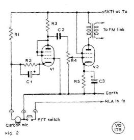
Fig. 2. Suitable FM modulator for the G3NBU two-metre Tx. Values can be: Cl, 10  $\mu$ F 25v.; C2. 0.1  $\mu$ F; C3, 25  $\mu$ F 25v.; R1, 22K one-watt; R2, 330 ohms; R3, 330K; R4, one megohm, control for deviation; R5, 330 ohms; T1, 1: 1 interstage, or two o/p xformers cascaded to give 1: 1; valves V1 EF91, or 277, 6AM6; V2, 6AQ5 or any similar audio pentode.
