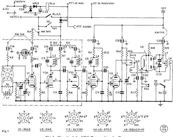
Fig. 1. Circuit of the VXO Transmitter for Two Metres by G3NBU.
