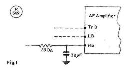
Fig. 1. Additional smoothing for hum elimination in the audio stage-see text.
