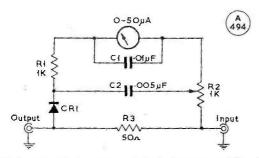
Circuit of the Antennascope, a simple but very useful aerial test item. C1, C2 should be disc ceramic; R1 is 3-watt, R2 linear carbon, non-inductive, and R3 carbon, rated at least one watt. Rectifier CR1 can be 1N34 or similar and the meter could be 0-100 <sub>IL</sub>A or higher—see text.
