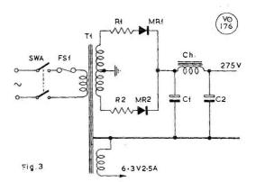
Fig. 3. Suitable PSU for the G3NBU rig. This is a standard arrangement, for which values could be: C1, C2, 50  $\mu$ F 450v. electrolytic; R1, R2, 100-ohm 6-watt wirewound; rectifiers MR1, MR2, BY127; smoothing choke Ch, 100 mA 10 Henry; mains xformer T1, 300v. each side, giving 125+ mA.
