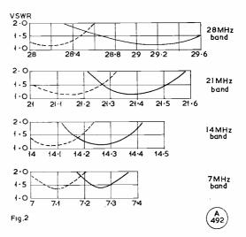
Fig. 2. VSWR curves to be expected with a properly dimensioned and connected 14-AVQ. Dotted lines are for the CW area, and solid line for the Phone coverage. These readings show why the favourite operating mode must be selected for best antenna response—see text. As it happens the CW coverage is nicely placed for most U.K. CW/SSB operators.
