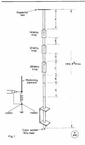
Fig. 1. Showing the layout of the Hy-Gain 14-AVQ trap vertical, element dimensions as given in Table I. The inset shows how the base of the aerial is fed across a coil embodied in the base section. As an additional protection a DC earth lead, of stout wire, should be connected with the radials, as indicated. The maximum overall length of the 14-AVQ, from coax connector to capacity hat, would be 19ft. 18‡ inches.
