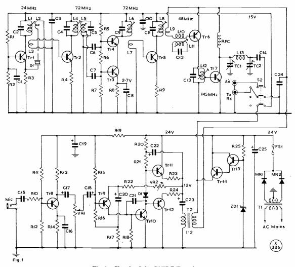
Fig. 1. Circuit of the G3TDZ Transistor Two-Metre Transmitter.
