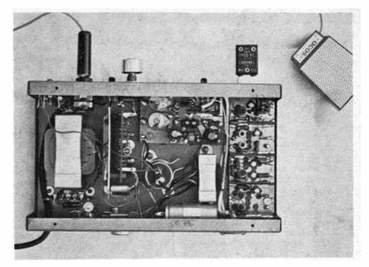
Transmitter as constructed by G3TDZ - underside view.
