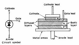
Fig.1. SYMBOL AND CONSTRUCTION OF A THYRISTOR
