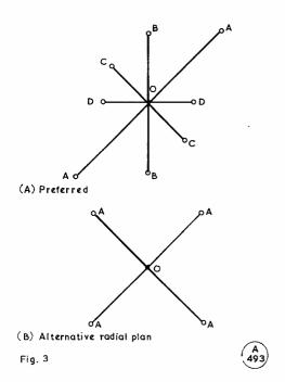
Fig. 3. Radial plans for the 14-AVQ. The 8-radial system at A is claimed to give superior results to the simpler arrangement at B. For both plans, dimensions are: 0-A, 33ft; 0-B, 16ft. 6in.; O-C, 11ft. 4in.; and O-D, 8ft. 4in. All measurements are from the base of the aerial to the insulator.
