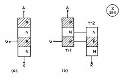
Fig. 2. TWO TRANSISTOR ANALOGY FOR A THYRISTOR
