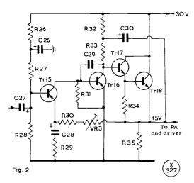
Fig. 2. Circuit for a series modulator for the Transistor Tx. — values in Table p.590.
