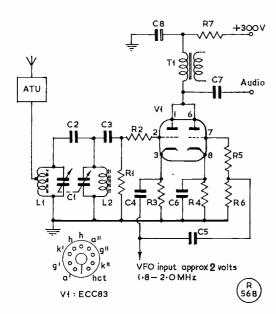
Circuit of Self-Balancing Heterodyne Detector for Top Band,
