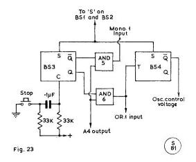
Fig. 23. Additional "stop" circuit that can be added to Fig. 22—see text.
