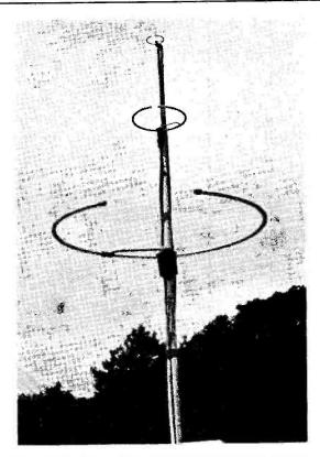
Whose is this? Seen at the Longleat Mobile Rally, a /M array for two metres, 70 cm. and 23 centimetres. We would very much like to hear from the owner, with a run-down on the gear.
