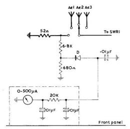
Fig.4. Diode RF voltmeter as alternative power indicator
