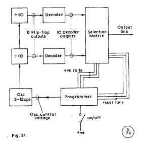
Fig. 21. Block diagram of the complete generator.
