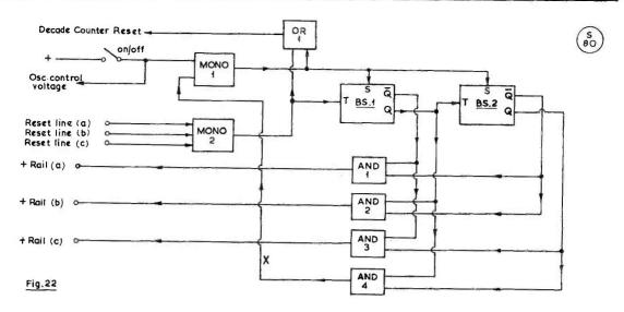
Fig. 22. Block diagram of simple CQ programmer-see text.
