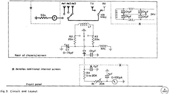
adhesive. The leads to the relay coil should be adequately screened, filtered and by-passed for RF.
