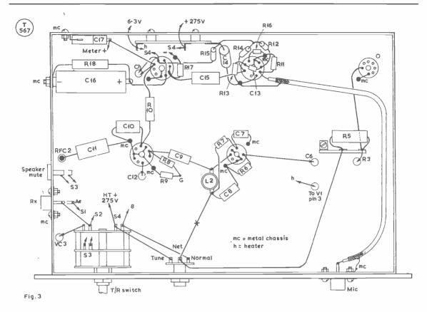
Fig. 3. Component layout and connections under-chassis.
