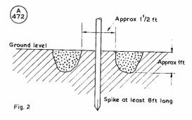
Fig. 2. To improve earth conductivity—of vital importance in installing an effective ground connection for a Top Band radiating system—fill the trench with rock salt or magnesium sulphate, then flood with water and cover with soil. Such an earth connection should be good for two or three years at least.
