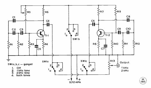
Fig. 3. Two-Tone Test Oscillator.
