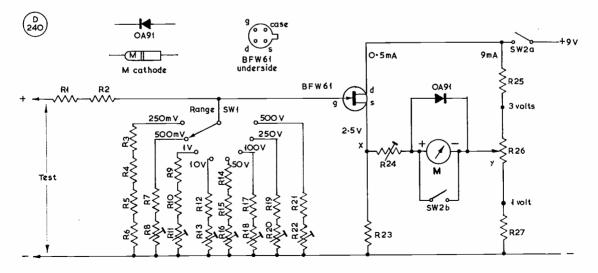
Circuit of the F.E.T. Voltmeter
