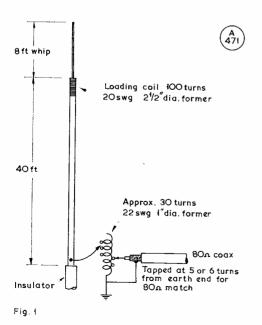
Fig. 1. Configuration for a top-loaded vertical system—see text.
