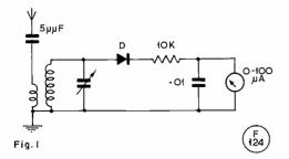
Fig. 1. Simple Harmonic Checker.
