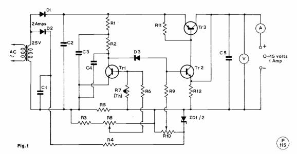
Fig. 1. Continuously Adjustable Fully Regulated Power Supply Unit.
