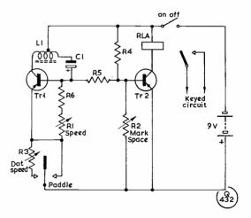
Circuit of the bug key described by G3PVH. The values he gives are: C1, 6 µF, 70v. working; R1, 100K variable; R2, R3, 5K variable; R4, 47K; R5, 10K; R6, 1:5K; Tr1, OC71; Tr2, OC72; relay, 4K coil resistance, to operate on about 2 mA. The feedback winding L1 is a valve-type output transformer, using only the centre-tapped primary.
