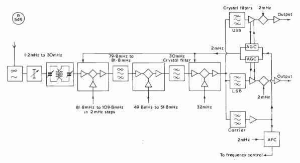
modulation products are better than 85 dB; cross-modulation -105 dB; and blocking -100 dB, referred to 1  $\mu$ V. In that part of the design specification dealing with cross-modulation, the requirement laid down was: "Without the use of aerial attenuation, with a wanted signal of 40 dB relative to 1  $\mu$ V and an unwanted signal of +105 dB, +105 kHz off-tune and modulated +105 dB, +105 kHz off-tune and modulated +105 dB relative to wanted output is permitted."
