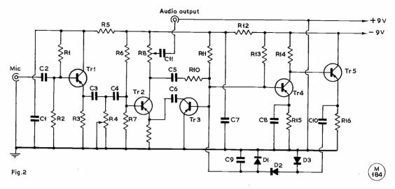
Fig. 2. Audio Peak Limiter for AM/SSB.
