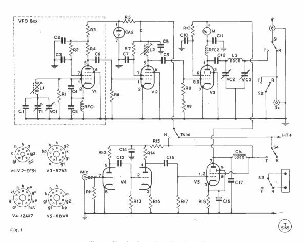
Fig. 1. Circuit of the Easy Top Band Tx.
