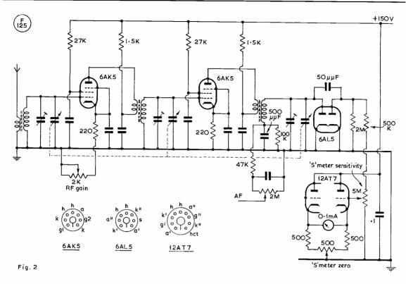
Fig. 2. Sensitive TVI Monitor-receiver.
