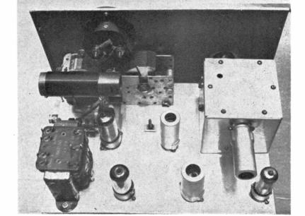
Inside rear view of the Tx, showing neat arrangement of the parts. PA tank coil L3 is at left and the VFO box on the right. The modulator choke is a speaker transformer—see text.
