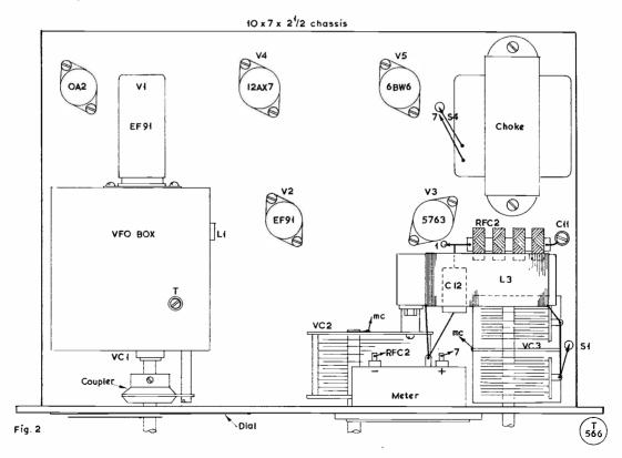
Fig. 2. Layout of the parts above chassis.
