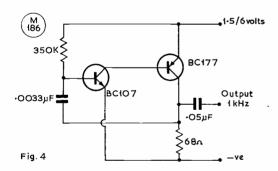
Fig. 4. Wide-band Signal Injector.
