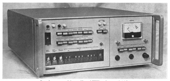
General appearance of the new Marconi H2900 receiver, covering 1.5 to 30 mHz, with a tuning accuracy to one cycle (1 Hz). The read-out as set in this picture shows that the Rx is tuned to a frequency of 17,603 kHz and 891 cycles (Hz). The applications of the H2900, a highly sophisticated design, are mainly military and commercial. In size it is only 22  $\times$  17½  $\times$ 71n. high, and its weight is 91 lb.
