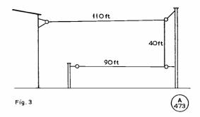
Fig. 3. Aerial configuration to get the high-current portion (the current antinode) into the vertical.
