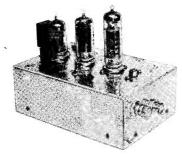
Constructed from a simple, trouble free, effective circuit, using obtainable valves ECC81, 6CH6, QQV03/10. Each unit is air tested and requires 250v. DC, modulated to PA and 250v. DC to supply the osc. and multiplier. Size  $6 \times 4 \times 2\frac{1}{2}$ .
