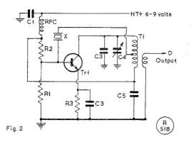
Fig. 2. New heterodyne oscillator, 7 mc, for Top Band operation with the Sommerkamp FT-100. Values are: C1, C2, 001  $\mu$ F; C3, C5, 100  $\mu$ F; C4, 3-5  $\mu$ F, trimmer; R1, 3.3K; R2, 33K; R3, 470 ohms, all half-watt; X, crystal 7+ mc, see text; T1, on §in. dia. Aladdin former with slug, primary 14t, 30g. tapped at 10th turn, secondary 3t. nearest to tap end; Tr1, n.p.n. transistor, 2SC372, or NKT10419. All built on board  $2\frac{1}{2}$ in. square—and see Fig. 6.
