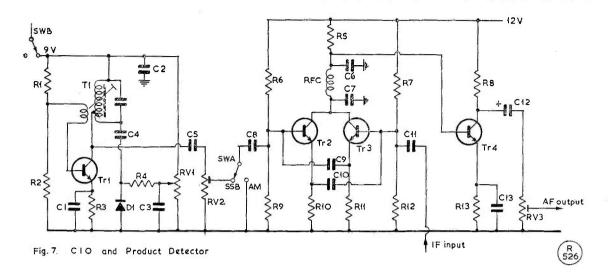
is very reliable.) All the general-purpose diodes show a change in self-capacity with applied voltage so it is not essential to use the rather expensive BA110—an OA202 seemed to work as well, but no long-term tests have been made. A buffer was originally fitted between the product detector and the oscillator but was found to be unnecessary. Unlike the old BFO system, a product detector does not require a high injection voltage.
