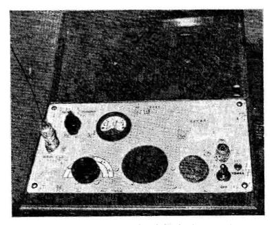
Interesting two-metre Transceiver, designed and constructed by G3VXZ (Maidenhead), and built into a standard metal (cash) box. The dimensions can be estimated from the size of the coax socket. The Transceiver can be operated from an external power source.
