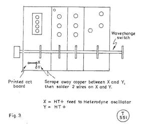
Fig. 3. Underside of the Sommerkamp FT-100 Transceiver—see text, p.278.
