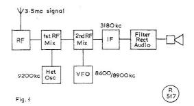
Fig. 1. Block diagram to show operation of FT-100 on 80 metres.
