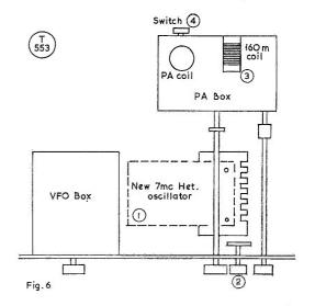
Fig. 6. Diagram to show how the FT-100 Top Band modifications are taken into the existing layout. (1), new 7 mc heterodyne oscillator; (2), change-over switch, see text; (3), 160m. PA coil, in series with 80m. coil; and (4), shorting switch, see text.
