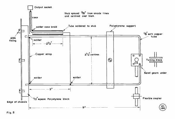
Fig. 5. The Pawsey stub output coupling for the Linear Amplifier.
