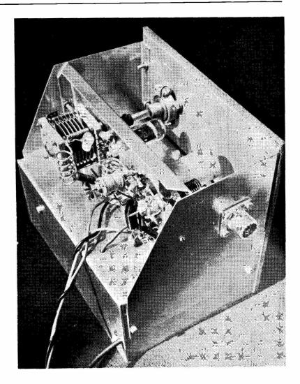
Another view of the constructional layout of the G3OGR two-metre converter—compare with drawings on p.218 and photograph, p.219. The socket on the near side of the supporting bracket is for aerial input—it could just as well be the standard-type Belling-Lee coax socket.
