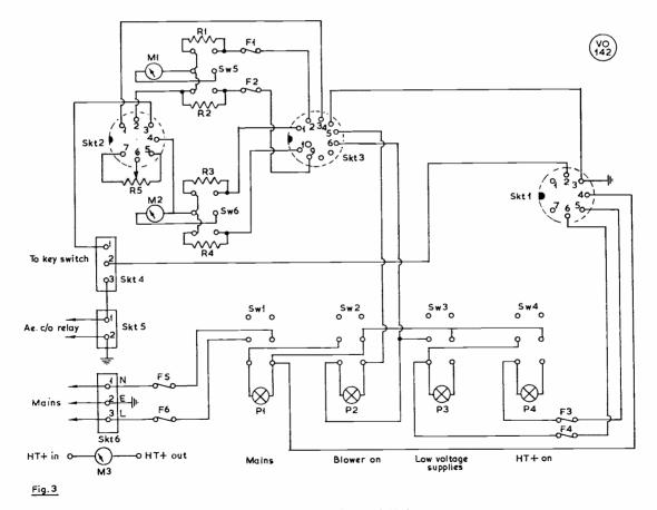
Fig. 3. Circuitry of the Control Unit-see text.
