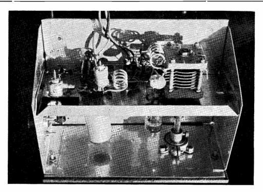
Construction of SEO two-metre Receiver.
