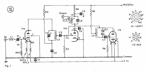
Fig. 1. Circuit of the SEO two-metre Converter
