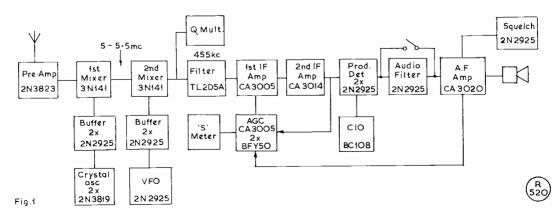
Fig. 1. Block diagram of the G3TDT Solid-State Receiver.
