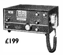
Unwanted sideband suppression is 45 dB, carrier suppression 60 dB, and distortion products are down approximately 30 dB.
