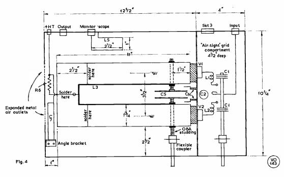
Fig. 4. General constructional layout of the Two-Metre Linear Amplifier—see text pp.222-223.
