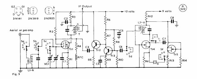
is the real answer. Some experiments were carried out on 10 metres. Without the pre-amp. and using a badly matched aerial strong broadcast signals were received that were traced (with a general coverage receiver) to the 17.5 to 18 mc band. This, of course, is the crystal oscillator *less* the first IF.
