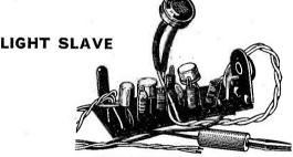
A light-operated mains switch turning on 1 kW electrical appliances automatically at dusk. Controls loads of up to 5A from a pre-set ambient light intensity.
