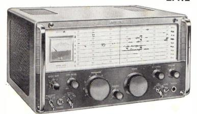
An amateur bands double-conversion superheterodyne receiver, for a.m, c.w, and s.s.b reception. For all amateur channels between 1.8 MHz and 30 MHz in nine 600 kHz bands with 28 MHz to 30 MHz in four bands.
