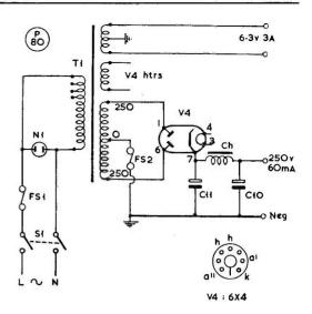
Fig. 4. Suitable PSU for the preselector—which could equally well be run from the main Rx power supply, if it has sufficient output capacity. Values are: C10, C11, 16 + 16 µF, electro-lytic; T1, 250-0-250v. 60 mA transformer, with necessary 6.3v. LT windings; Ch., 5 Hy 100 mA LF choke; V4, 6X5G or similar rectifier: F1, 750 mA mains fuse; F2, 100 mA antisurge fuse.
