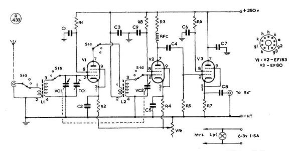
Fig. 1. Circuit of the three-stage RF preselector, with V1, V2 as gang-tuned amplifiers and V3 as a cathode follower to give a good match, through 75-ohm coax line, into the front end of almost any receiver.
