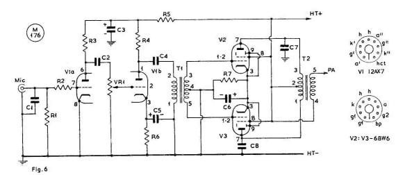
Fig. 6. Push-pull Modulator for a Crystal Microphone.
