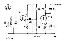
Fig. 12. Solid-state arrangement for a two-metre RF stage, by G3BKQ.
