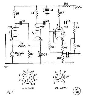
Fig. 8. Carbon microphone amplifier needing neither transformer nor valve phase-splitter.
