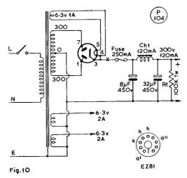
Fig. 10. A suitable power supply circuit for the Top Band transmitter circuits shown in the article by G3OGR.
