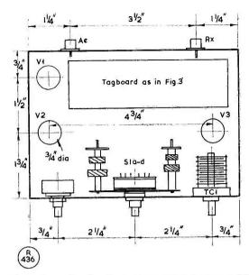
Fig. 5. General under-chassis layout sketch. The assembly is 6in. long by 4in. wide by 2½in. deep, and the front panel (not shown) is 7½in. long by 5½in. deep.
