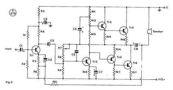
Fig. 11. Transformerless Audio Amplifier, solid-state.
