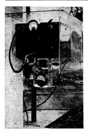
View of the ATU as mounted for convenient operation out-ofdoors. It loads into a vertical radiator—see text and accompanying circuit diagram.
