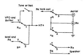
Fig. 9. Switch for Transmit/Receive
