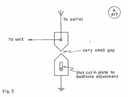
Fig. 5. Construction of a simple but effective static-discharge gap—see text.
