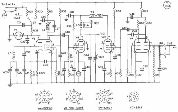
Fig. 8 TRANSMITTER SECTION
