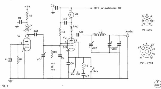
Fig. 1. Circuit of crystal-controlled Top Band transmitter.
