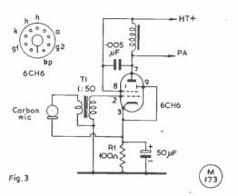
Fig. 3. An "economy" (or simplified) single-stage modulator, for a carbon microphone.
