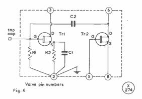
Fig. 6. Mixer and oscillator module, to replace 6K8. C1, .001  $\mu$ F; C2, 3-5  $\mu\mu$ F; R1, 1 megohm; R2, 10K; Tr1, 2N3819 or MPF105; and Tr2, MPF104 or 105.
