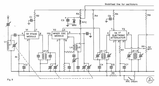
Fig. 9. Modified BC-454 receiver, showing modules as follows: V1, RF stage; V2, mixer losc.;
