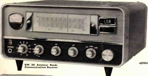
The KW201 is now being manufactured with 2 detectors (i) product detector for SSB and CW (ii) diode detector for AM. The KW201 has been specifically designed for optimum performance on SSB. 11 ranges give coverage 1.8 mc/s. to 30 mc/s. A mechanical filter gives an IF selectivity of 3.1 kc/s. at 6 dB, and 6 kc/s. at 60 dB. A "Q" multiplier is available giving a variable range of 3.1 kc/s. to 200 cycles selectivity.
