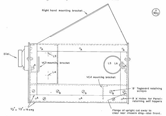
Fig. 7: ELE VATION ON TRANSMITTER SIDE - side panel removed
