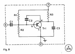
Fig. 8. The Vacar circuit BFO module, excellent for short and long-term stability and specially suited to single-frequency working. C1 is 100  $\mu\mu$ F; C2, C3, .001  $\mu$ F; R1, 4.7K; R2, 10K; R3, 2.2K; and Tr1, OC170/171.
