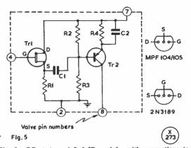
Fig. 5. RF stage and 2nd IF module, with connections to replace a 6SK7 valve. Values are: C1, C2, 001 μF (C2 for a 2nd IF only); R1, 3.3K; R2, 22K; R3, 100K; R4 (RF stage only), 1K; R4 (2nd IF only) 330 ohms; Tr1, 2N3819, MPF104 or MPF105; and Tr2, OC170/171.
