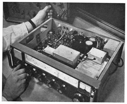
The new Eddystone 990R is claimed to be one of the most versatile and compact VHF (27 to 240 mc coverage) receivers ever designed. It is completely solid-state, suitable for mobile, portable or fixed-station operation in a variety of applications over the metre bands and, though a mains PSU is built in, it can be run directly from a battery supply if required.
