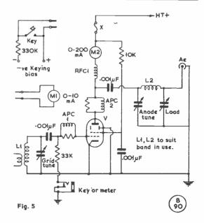
loading and redipping may be repeated until the stage is "loaded up" to the point where the anode current on the meter at the bottom of the dip is as desired. HT may then be switched off, and the dummy load replaced by an aerial. If the aerial departs appreciably from the 75-ohm characteristic, (so that the feeder has standing waves on it) it will almost certainly be necessary to "touch up" the tuning of the PA tank circuit to some slight extent.
