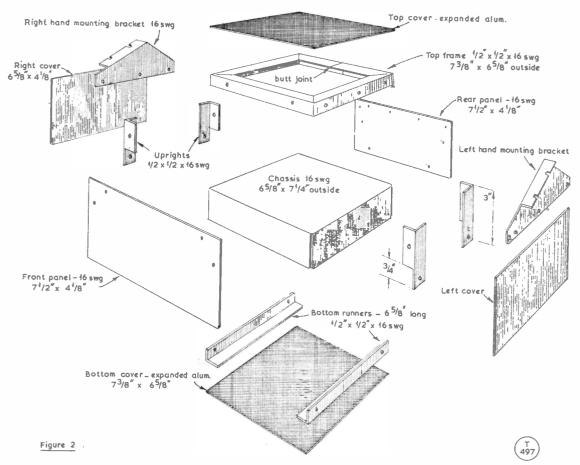
Fig. 2. Some main constructional details — see text.
