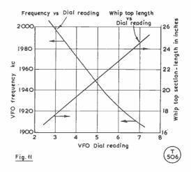
Fig. 11. Calibration curves obtained on the G3SFL/M equipment—see text.
