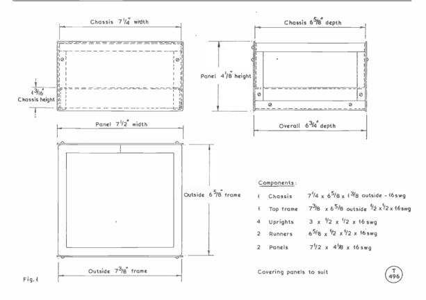
Fig. 1. General mechanical design for the G3SFL/M rig.
