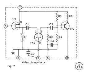
Fig. 7. First IF amplifier with electronic attenuator. Values: C1, C3, C4, .001  $\mu F$ ; C2, .002  $\mu F$ ; R1, 3.3K; R2, 8.2K; R3, 22K; R4, 100K; R5, 1K; T1, 2N3819; Tr2, MPF104; and Tr3, OC170/171.
