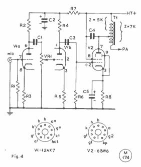
Fig. 4. Class-A modulator for use with a crystal microphone—values are given above.
