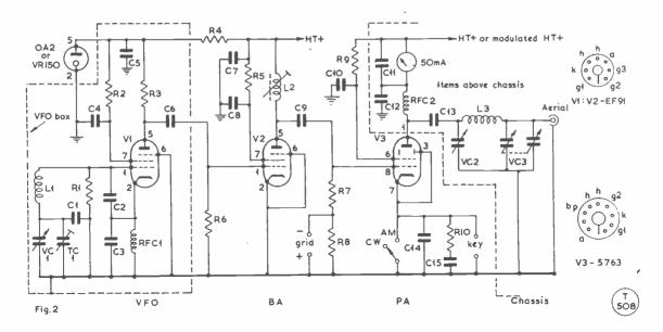
Fig. 2. Three-stage VFO controlled 160m. transmitter.
