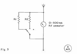
Fig. 3. An aerial RF ammeter can be shunted if the range is not right for some bands, depending on aerial impedance and therefore current. R1, R2 can be made from fire-element wire.
