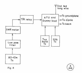
Fig. 4. The order in which the items should be inter-connected to make full use of the ATU assembly described in the article.
