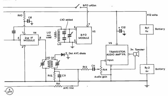
V3. 1st IF and attenuation, V4. 2nd IF; V5, BFO module; and V6, transistor amplifier.
