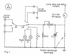
Fig. 1. Circuit diagram of the unit, S1 is the input selector switch and S2 the output. R is 80-ohm high-wattage carbon, L a rotary-roller type tuner (see text) and C is 200  $\mu\mu\text{F}$ , widespaced.
