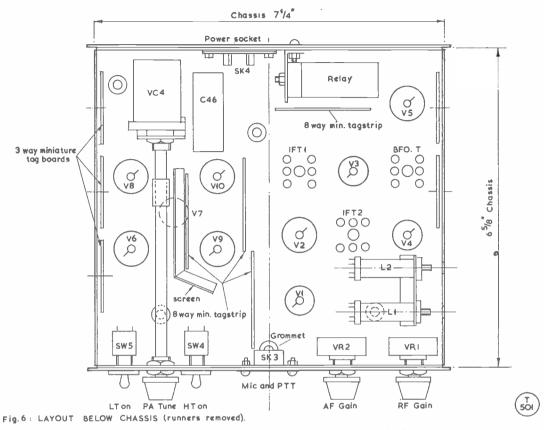
Fig. 6 (Above) the under-chassis layout. Fig. 10. (below) Heater connections and control circuitry.
