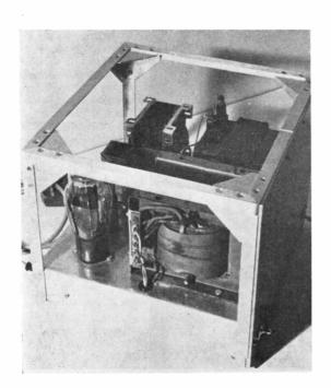
Example of intergrated case-chassis construction, as applied to the PSU for the G3SFL/M Tx/Rx. The weight of the unit is about 30 lbs., and it can be lifted by holding the centre of any one of the three open sides of the top frame.
