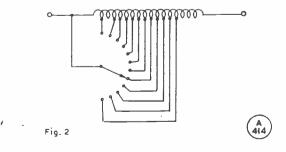
Fig. 2. A simple alternative to the rotary-roller type of inductance—a tapped coil with a low-loss 12-way switch to short out unwanted turns.
