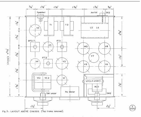
Fig. 5. The layout above chassis—and see Fig. 6, p.744.
