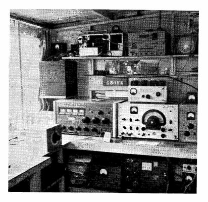
Hector Cole, G3OHK, 25 Causeway Road, Seaton, Workington, Cumberland, runs a home-built SSB Tx (left), with a kit-constructed K.W. Victor (extreme right) and has a variety of auxiliary items, including gear for two metres. The HF-band aerial is a 135ft. wire. The receiver at centre is also a home-built job for all-band coverage.
