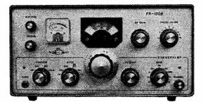
FR-100B double conversion superheterodyne with crystal controlled first mixer, 80-10 metres £112 0 0
