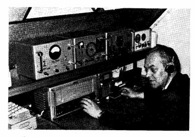
The station of Fritz Cramer, DL3MO, 4420 Coesfeld, Schuppenstrasse 22, Westphalia, near the Dutch border. Fritz started on the air in 1949, runs CW with an electronic key, and AM phone. The Tx is a home-built five-band job covering 10 to 80 metres, with a multi-band dipole outside.
