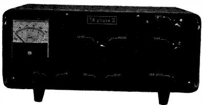
Drive Frequency: 28-30 mHZ. SSB or A.M. Drive Power: 10-200 watts.
