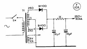
Fig. 2. Circuit and values for a power supply unit suitable for the instrument described in the text. It should give 50 mA or so at 250v.
