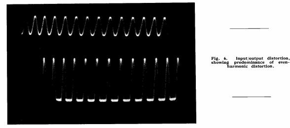
cycle only shows the point even more clearly, and demonstrates the non-coindicence differing by some degrees over  $180^{\circ}$ . There is evidence that the half-wave is not perfectly sinusoidal as compared with the previous picture. This is undoubtedly due to excessive amplification on the Y-plate amplifier in order to obtain a sizable display, and is a well-known feature in many oscilloscopes, demonstrating the precautions that must be taken in order to obtain a faithful trace.
