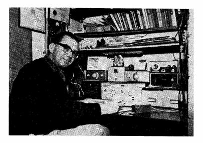
The station of G3HTB, Malcolm Squance, 57 The Drive, Alwoodley, Leeds 17 has been shown in "Short Wave Magazine" before in April 1955. Since then, many changes have been made, the rig pictured here consisting of a Codar-66 with PR-30X, RQ-10 Q-multiplier and AT-5 transmitter—in fact, an all-Codar station, which gives good results.
