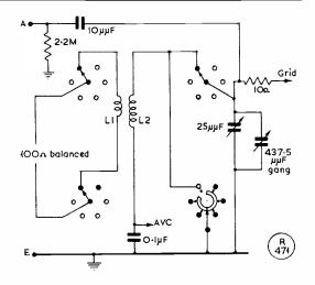
between frequencies and scale markings. Band 4 can be aligned at 1.9 mc and 3.7 mc; Band 5 at 5 mc and 10 mc; and Band 6 at 14 mc and 28 mc. [cont'd over
