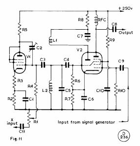
Fig. 11. Typical Wobbulator circuit, for which values can be: C1, C6, C7, C10, C11, 0.1  $\mu$ F; C2, 30  $\mu\mu$ F trimmer; C3, C4, C8, C9, 50  $\mu\mu$ F; C5, to tune L1, L2 to about 5 mc; R1, 1-meg. pot.; for sweep width; R2, about 150-450 ohms; R3, about 150 ohms; R4, 470K; R5, R10, 4.7K; R6, 47K; R7, about 150-450 ohms, R8, 18K; R9, 27K; V1, small RF pentode; V2, ECH81 or similar. L1, L2. to tune 5 mc. Experiment with R2, R3 and C2 values for best sweep and linearity with valve used.
