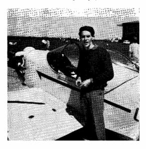
G3NRB (Datchworth, Herts.) arrived for the Alconbury Rally in his smart little "Turbulent" aircraft, G-AJCP. It is in the ultra-light category, for short-range flying, with an endurance of about two hours, and is powered by a 28 h.p. modified Volkswagen engine.
