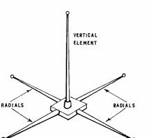
Fig. 3. Construction of a typical ground-wave aerial.
