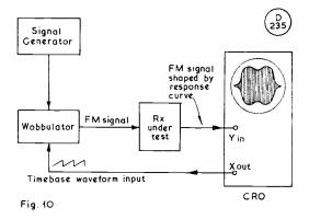
Fig. 10. Layout of equipment for checking frequency response —see text.
