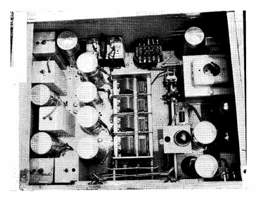
Looking inside the CR-100. The valves adjacent to the tuning gang, from the rear, are (1), 1st RF; (2), 2nd RF; (3), mixer; and (4), oscillator. Valves from front left to back are (1), 1st IF; (2), 2nd IF; and (3), 3rd IF. At right, the BFO stage, DDT AF, output and rectifier stages. The noise limiter double-diode is on a bracket over the aerial trimmer extension shaft. At the back, from right to left, are the smoothing components, output transformer and audio filter.
