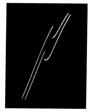
Fig. 3. A tunnel-diode trace showing the bi-stable regions.
