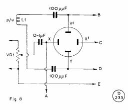
Fig. 8. Circuit for modulation monitoring, to produce the pictures shown in Fig. 9. L1 is a small link coil coupled to the PA tank such that sufficient RF can be fed to the Y-plates. VRI is one megohm, connected across the modulator to get about 50-100 volts of AF, and fed via a suitable HV condenser. Points A, B, C and D go to the shift controls on the 'Scope. L1 must be insulated to prevent HT contact and can be tuned if RF pick-up is insufficient.
