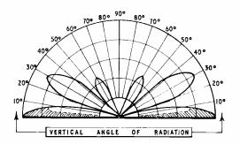
Fig. 2. Lobes and radiation angles of a vertical half-wave dipole centred a full wave above ground. Shaded portion below 5° indicates no radiation due to ground losses. Note (a), reduced power in ground-wave lobe at 8° compared to Fig. 1; (b), major radiation occurring at 30°, and (c), formation of a further lobe at  $60^\circ$ .
