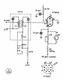
Fig. 1. Cathode tuning meter for the CR-100.
