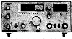
NCX5 Mk. 2 Top Quality Transceiver. 80-10 ; 200W p.e.p.; SSB/CW/AM. £225 less p.s.u. (p.s.u. kit £25)
