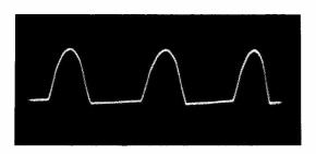
Fig. 2. Trace when using half-wave rectification, with some evidence of reverse current.
