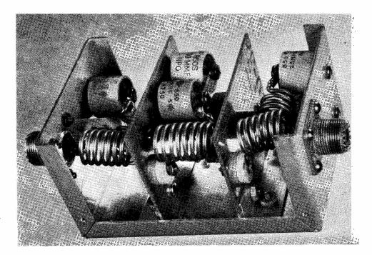
An impression of the Low-Pass Filter, as built by the author and described in the text. The circuit and values are given with the diagram, and it should prove an efficient aid for TVI suppression.
