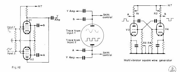
Fig. 12. The basic circuit for a beam-switching unit. Depending on the type of valve used for V1, V2, they can be switched either on the screen, the suppressor or control grid; a frequency-changer type of valve will give best results. For V3, V4, pentodes are recommended, to give least distortion of the traces. R1, R2, is a 50K two-gang separation control, and R3, R4, a two-gang 500K speed control.
