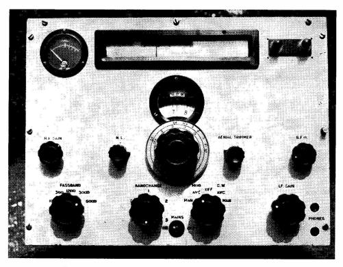
Front appearance of the CR-100, with the tuning meter fitted to the left of the horizontal window, in which appears the band selected by the wave-change switch. The terminals on the other side of this window provide HT/LT for accessories, such as a crystal calibrator. The circular dial carries the amateur-band markings, in addition to the existing internal geared-drive scales. The modifications involved are discussed in the article by G30GR.
