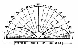
Fig. 1. Lobe and radiation angle of a vertical half-wave dipole with its centre a quarter-wave above ground. Shaded portion below about 5° indicates no radiation due to ground losses. While peak radiation occurs at around 10°, overall radiation  $\pm 3$  dB is between 5° and 30°.
