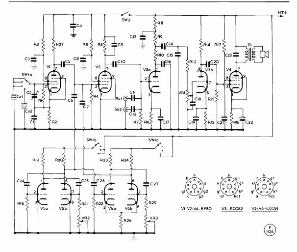
Fig. 1. Circuit of the Crystal Calibrator-Heterodyne Frequency Meter, in which VI is the master oscillator and V5, V6 are triode-connected multivibrators, giving respectively 100 kc and 10 kc beats. V2 is an amplifier to ensure good harmonic output. V3A is a mixer for external inputs, such as a signal generator. V3B, V4 are audio amplifier stages, enabling a speaker to be driven for bench work.
