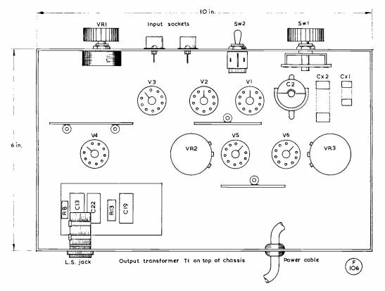
Fig. 3. Showing the general layout as adopted for the prototype, on a standard chassis 10in. by 6in. wide with a 2in. sub-space. Some constructional points are covered in the text.
