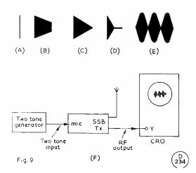
Fig. 9. The traces to be expected when checking modulation —see text. A two-tone test signal trace is shown at (E), and (F) is the set-up for SSB Tx testing when using the recommended two-tone input method.
