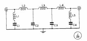
Circuit of the LPF as described and illustrated, for which values can be: C1, C4, 50  $\mu\mu$ F ceramic; C2, C3, 150  $\mu\mu$ F ceramic; L1, L5, four turns 14g. wound to  $\frac{1}{2}$  In. i.d., spaced at 8 t.p.i.; L2, L4, seven turns, ditto; and L3, 8 turns.
