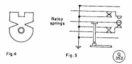
Fig. 4. The isthmus armature—see text. Fig. 5. A contact configuration to give change-over operation when used with coaxial cable. This kind of motion can be built up by manipulating contacts suitably. It is simply a matter of careful examination of the available spring-set parts.
