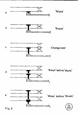
Fig. 3. Showing some possible arrangements of contacts on a GPO relay. When bought as surplus, almost any contact configuration may be encountered.
