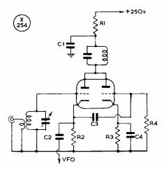
Fig. 1. Circuit of a balanced-mixer arrangement suitable for preventing VFO break-through into the IF strip. Values are: C1, C4, 01  $\mu F$ ; C2, 001  $\mu F$ ; C3, 220  $\mu \mu F$ ; R1, R4, 100K; R2, 2.2K; R3, one megohm. See text for discussion.
