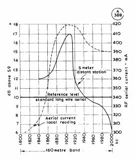
Fig. 2. With the arrangement shown in Fig. 1, resonated at a suitable Top Band frequency, these curves were plotted under practical test conditions, in co-operation with another 160m. station 15 miles away. With the system resonated at 1900 kc, the bandwidth for VFO operation would be good enough over 1880-1920 kc. The dotted line shows how closely the Tx aerial current followed the S-meter reading at the distant station.
