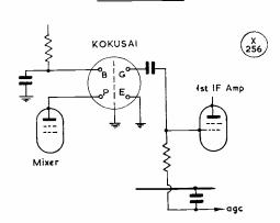
Fig. 3. Circuit for replacing an IF transformer with the Kokusai mechanical filter.
