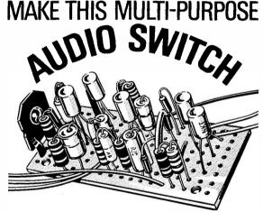
. . . from full instructions in the May PRACTICAL WIRELESS. Assembled on Veroboard this 5 transistor unit can switch on or off a radio, TV, lighting, heating, tape recorder, dictation machines, etc., up to a range of 30ft. by audible means.
