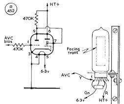
Fig.t: Circuit and layout for EM84 tuning indicator
