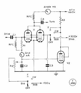
Fig. 2. Modified 807 PA, as Fig. 1, for CW, SSB or AM working at will. CI is as normally used on the PA grid side; C2, 0.1 µF; C3, C4, as normally used; R1, 10K; R2, 10K control potentiometer, see text; R3, as for screen dropper under AM/CW conditions; switching can be by using a ganged Yaxley-type arrangement.
