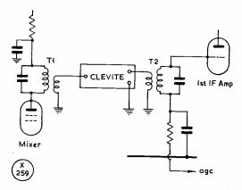
Fig. 6. The Brush-Clevite ceramic filter can be used with a valve receiver to achieve better selectivity. If plenty of gain is already available, T2 can be omitted—see text.
