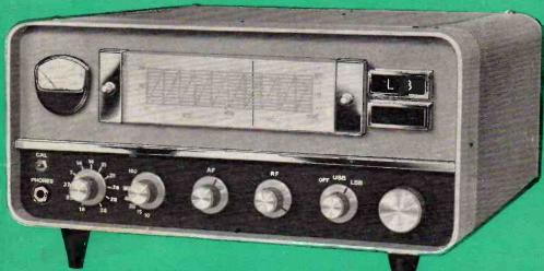
The KW 201 has been specifically designed for optimum performance on Single Sideband. Il ranges give coverage in the amateur bands from 1.8 mc/s. to 30 mc/s. A mechanical filter gives an I.F. selectivity of 3.1 kc/s. at 6 d.b., and 6 kc/s. at 60 d.b. A 'Q' multiplier is available giving a variable range of 3.1 kc/s. to 200 cycles selectivity.
