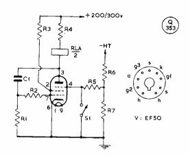
As explained in the text, with the values given here a 40-second pause can be obtained before the relay answers. Since the delay is controlled by Cl, Rl, it is variable over wide limits—see text.
