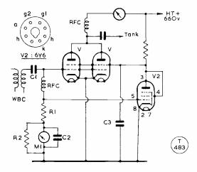
Fig. 1. A typical RF power amplifier circuit using a pair of 807's in parallel, with V2 as the clamper. The usual pi-network tank is assumed.
