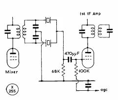
Fig. 2. Method of connecting a half-lattice filter into a receiver. Several sections can be cascaded to give better rejection of unwanted signals.
