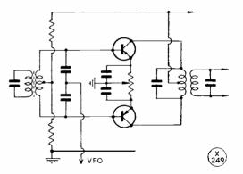
Fig. 9. Balanced mixer using two transistors.
