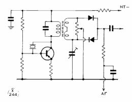
Fig. 4. More conventional method of feeding the balanced modulator.
