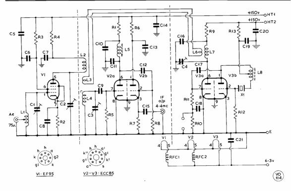
Circuit complete of the four-metre converter, by G3TDR, discussed in the article. Basically, it is a straight-forward valve design, the idea being to achieve reasonable efficiency using readily-obtainable parts, to enable anyone not having any gear for four metres to get going with a good first converter. It is a crystal-controlled arrangement, with the IF side tuned across 4.1 to 4.7 mc to cover 70.1-70.7 mc at signal frequency.
