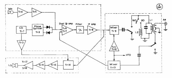
Fig. 1. Block diagram of experimental transistor transceiver.
