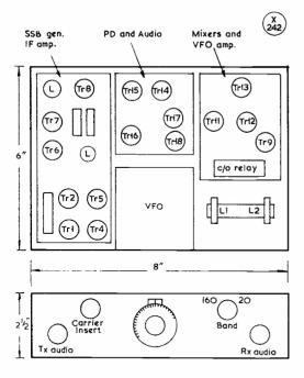
Fig. 2. Layout of experimental transceiver.
