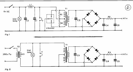
There are various ways of getting the Class-D Wavemeter (designed in the original for 6-volt DC input) to work off AC mains. This is the safe way of doing it. Fig. 1 is the circuit before modification, and Fig. 2 shows the final arrangement. Values are, for Fig. 2: C3, 0.1  $\mu$ ; C4, C5, 8  $\mu$ F; R3, 1000 ohms; T1, existing vibrator transformer; and T2, heater transformer using 6.3-volt secondary as 6-volt AC input into original rectifier-smoothing section.
