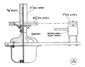
Cross-section view of the rotator, made from bits-'n-pieces ---windscreen-wiper motor (ex-junk yard, 2s. 6d.), and parts from a discarded vacuum cleaner (see text).
