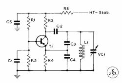
Fig. 13. Using an OC171 as a Colpitts VFO in the groundedbase circuit. C2 should be selected as the smallest value to maintain oscillation and in any case should not be greater than 47  $\mu\mu$ F. Other values, for 8 mc, are: C1, C5, 0.1  $\mu$ F; C3, C4, .001  $\mu$ F; VC1, 75  $\mu\mu$ F; R1, R3, 4.7K; R2, 680 ohms; R4, R5, IK; L1, Denco D.P. Range 5, blue; and transistor OC171.
