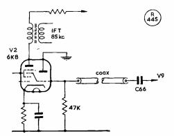
Fig. 2. The second frequency-changer. Components are mainly as shown around V2 in the S.640 manual — and see text.
