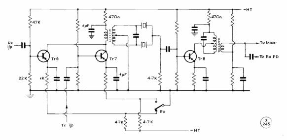
Fig. 5. IF Strip of experimental transceiver.
