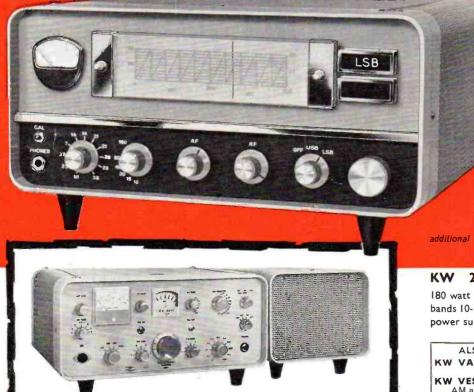
The KW 201 has been specifically designed for optimum performance on Single Sideband, 11 ranges give coverage in the amateur bands from 1.8 mc/s. to 30 mc/s. A mechanical filter gives an I.F. selectivity of 3.1 kc/s. at 6 d.b., and 6 kc/s. at 60 d.b. A 'Q' multiplier is available giving a variable range of 3.1 kc/s. to 200 cycles selectivity.
