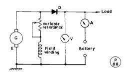
Circuit using diode limiter.
