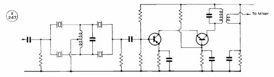
Fig. 7. Alternative IF strip using a cascode amplifier.
