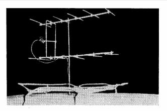
The mobile 70-cm. array carried on his car by G8APX (Witnesham, Ipswich) is a 6-over-6. The position of this beam has been found by trial-and-error for optimum radiating efficiency. The Tx runs 6 watts, and some very satisfying results are being obtained on the 430 mc band. During April, G8APX will be touring Scotland and would like to fix skeds with anyone up there.
