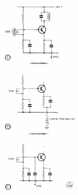
Fig. 8. Single-ended mixer configurations.
