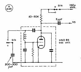
Fig. 3. Using the Electroniques HSO-85 oscillator unit as the 85 kc BFO for the S.640. The switch SIA-B, a double-pole three-way rotary, can occupy the panel position formerly taken by the BFO on-off switch.
