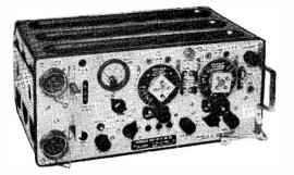
This set is made up of three separate units :--(1) a two valve amplifier using a 6V6 output valve; (2) (some only) a V.H.F. transreceiver covering 229-241 Mc/s. using 4 valves; (3) the main
