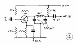
Fig. 11. The product detector used in the experimental transceiver.
