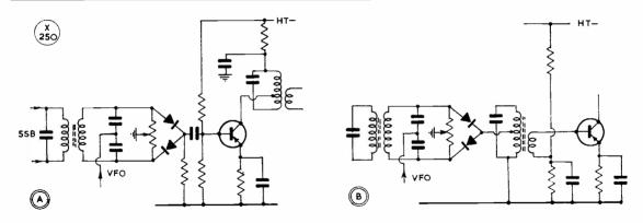
Fig. 10. An economical balanced mixer using two diodes followed by a single stage of amplification. Circuit (B) is preferred.
