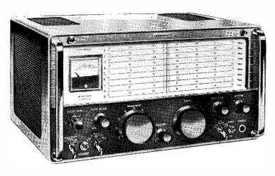
An amateur bands double-conversion superheterodyne receiver, for a.m. c.w. and s.s.b reception. For all amatechannels between 1.8 MHz and 30 MHz in nine 600 kHz bands with 28 MHz to 30 MHz in four bands
