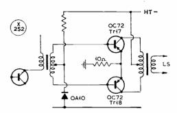
Fig. 12. Audio output stage with temperature compensation.
