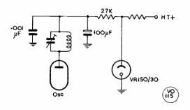
Simple splatter-suppression circuit.
