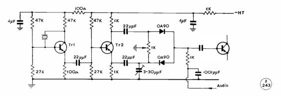
Fig. 3. Carrier oscillator and balanced modulator used in experimental rig.
