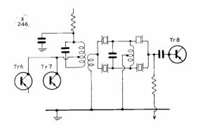
Fig. 6. Method of matching into a two halflattice section filter.
