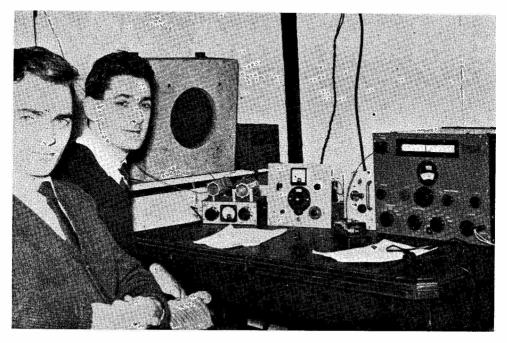
Batting for North Notts, and signing G3RCW were G3NHE (left) and G3PRD. Their gear consisted of G3NHE's home-built transmitter (left) running 10 watts to a PL81 as PA, the receiver being a CR-100 and the aerial "about 120 feet of wire," end-fed through an ATU. With this rig they made 508 points to put them into 11th place out of more than 90 entries.
