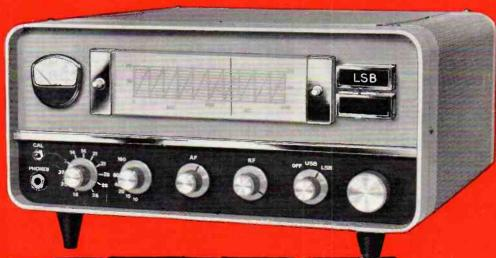
The KW 201 has been specifically designed for optimum performance on Single Sideband. Il ranges give coverage in the amateur bands from 1.8 mc/s. to 30 mc/s. A mechanical filter gives an 1.P.a selectivity of 3.1 kc/s. at 6 d.b., and 6 kc/s. at 60 d.b A 'Q' multiplier is available giving a variable range of 3.1 kc/s. to 200 cycles selectivity.
