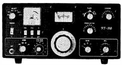
FT-100 transistorised transceiver, 150 watts s.s.b./c.w./a.m., 10-80 metres (28-28-5 mcs. + 4 Xtal channels), 50-75 ohm, double conversion, better than 1 uV for 10 dB S/N ratio, built-in 100 kcs. Xtal cal., 1 rev. = 50 kcs., 2·1 kcs. at 6 dB, 2·5 kcs. at 60 dB, built-in power supply 110/220v. a.c./12 d.c., needs 10 watts on receive, 200 watts on transmit, provision for VOX, only three tubes, driver 12BY7, 2 x 6JM6 p.a., width 13", height 6", depth 10", weight 40 lbs. £180
