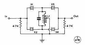
Fig. 6. Circuit for improved crystal filter, in which X1=X3, and X2=X4. For frequencies see text Part I. Inductance L1 in this circuit can be of 55 turns, centre tapped, shunted by 47  $\mu\mu$ F.
