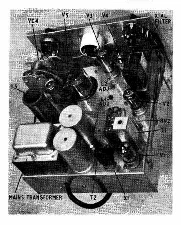
Identifying the positioning of components above chassis.
