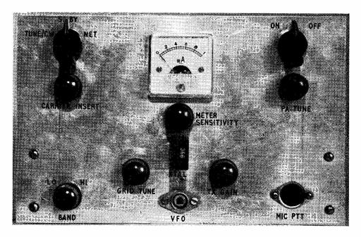
Front-panel view showing layout of controls for SSB Exciter as described in the article.
