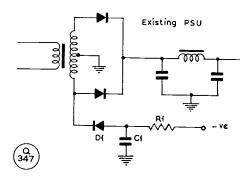
Fig. 2. Using the existing Tx PSU to get power for the T/R Switch. C1 is 6  $\mu F$ , 350v. DC working ; R1 can be 10K 2-watt but should be adjusted to give 200v.; and D1 is a 500v., 100 mA rectifier.
