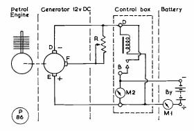
Key to the G3CGQ P-E arrangement: D, dynamo; F, field winding; E, body of generator; control box rheostat R, 10 ohms, 20w.; cut-out, from any 12v. car with pos. earth system; control box connections, D to D on generator; B to 12v. battery neg., E to earth, battery pos. and body of generator; meter M1 0-20 amp., M2 0-20 volts; Lattery 12v. 80 amp. hour.
