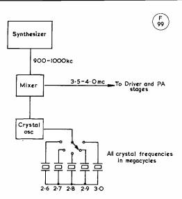
Fig. 2: Simple method of extending range of basic 3 decade system
