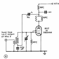
Fig. 7. PA configurations suitable for the "Mini-5". (B) is the preferred method of feeding and should be neutralised as shown. With a pair of 807's, or 5B254M's, in parallel something like 100 watts output can be realised with an HT supply of 1000v.
