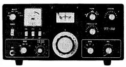
FT-100 transistorised transceiver, 150 watts s.s.b./c.w./a.m., 10-80 metres (28-28-5 mcs. + 4 Xtal channels), 50-75 ohm, double conversion, better than 1 uV for 10 dB S/N ratio, built-in 100 kcs. Xtal cal., 1 rev. = 50 kcs., 2-1 kcs. at 6 dB, 2-5 kcs. at 6 dB, built-in power supply 110/220v. a.c./12 d.c., needs 10 watts on receive, 200 watts on transmit, provision for VOX, only three tubes, driver 12BY7, 2 x 61M6 p.a., width 13", height 6", depth 10", weight 40 lbs. .... £180
