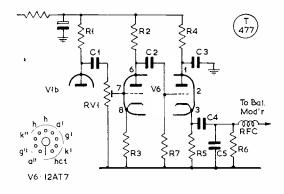
Fig. 5. Alternative audio section—see text. Values are: C1, C2, C3, C4, 0.5  $\mu F$ ; R1, R2, 100K; R3, R4, R6, 1K; R5, 2.2K; R7, 470K; RV1, 470K potentiometer, gain control; V6, 12AT7.
