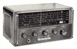
be successfully resolved by appropriate setting of the BFO for carrier reinsertion. A total of 13 transistors and diodes is used, leading to high sensitivity and consistent results on all ranges. The main scales occupy a length of nine inches and are clearly calibrated direct in frequency. The standard Eddystone precision slow-motion drive controls the tuning, which is exceptionally smooth and light to handle. An auxiliary logging scale permits dial settings of chosen stations to be recorded.
