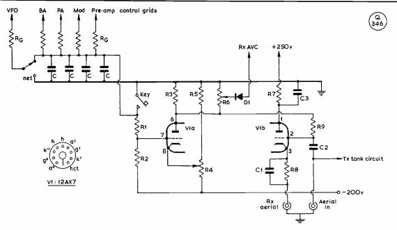
Fig. 1. Circuit of the T/R switch, for which values can be : C1, .0015  $\mu$ F; C2, 500  $\mu\mu$ F; C3, .01  $\mu$ F; R1, R2, R3, 100K; R4, 10K pot.; R5, 20K, 2w.; R6, 500K pot.; R7, 50K; R8, 2.2K; R9, 1 megohm. RG are existing grid resistors; condensers C are .001  $\mu$ F, decouplers; D1 is a germanium diode, GD3 or similar, and the valve is a 12AX7.
