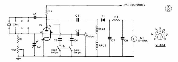
Fig. 1. Circuit of the Test Oscillator.
