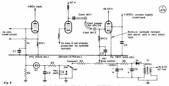
Fig. 2. Suitable modifications for any AM/CW Tx to allow for use of the SB10 Sideband adapter. A time-sequence, grid-block keying circuit is also shown, the SB10 then controlling the "send-receive" switching via the key-jack. If necessary, the driver can also be included in the grid-block keying circuit if it is not already protected with cathode bias during stand-by.
