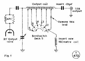
Fig. 1. Modification to put the SB10 output tank circuit (10-metre section) on to 160 metres — see text.
