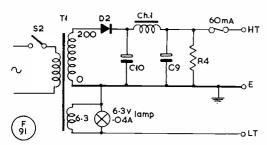
Fig. 2. A Suitable PSU for the Tester.
