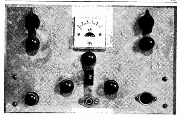
Front panel view of the G3RNL Sideband Exciter | Transmitter
