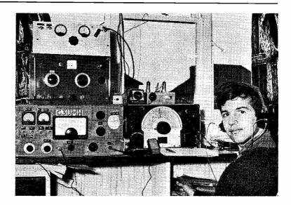
Station of Alan Dailey, G3UMH, of 1018 York Road, Leeds, 14. He has been on the air for 13 months, starting off on 160m., but is now mainly active on 21 mc, CW and Phone, running 50 watts and a dipole. The equipment includes two transmitters, one a xtal/mixer type for 14-21 mc CW, and the other covering 10-80m., CW/AM, using a 2-match coupler; he also has an HF-band crystal converter as a front-end feeding into the R.1155 Rx.
