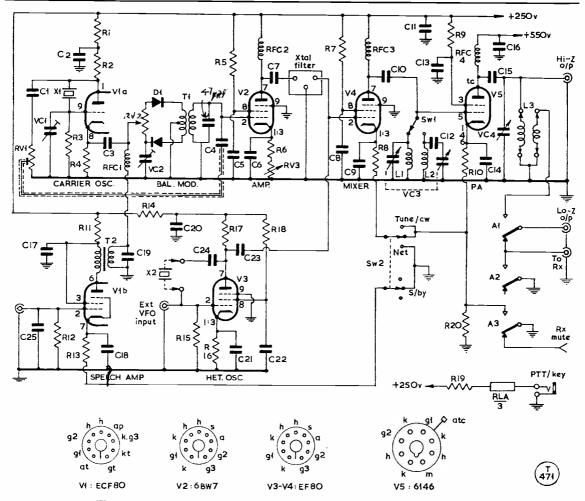
Fig. 1. Circuit of the Five-Stage All-Band SSB Exciter | Transmitter
