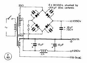
Fig. 2. Suitable PSU for the Tx, using BY100's in bridge to get +550v. from the 250-0-250v. transformer, rated 100 mA.
