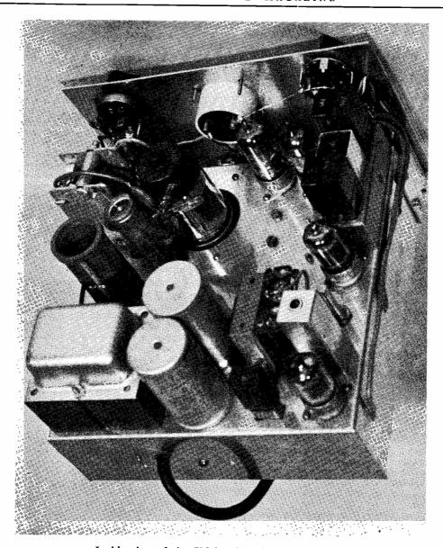
Inside view of the Sideband Exciter | Transmitter
