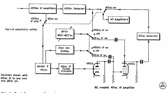
Fig. 3. Beat Frequency Heterodyne System for Dual IF Operation, Bands 3-18 only-see text.
