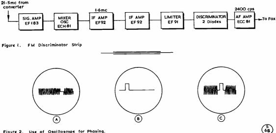
Figure 2. Use of Oscilloscope for Phasing.
