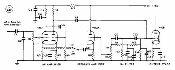
Fig. 2. Circuit of the R.C.A. AR-8516L Feedback Amplifier.
