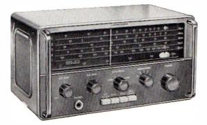
be successfully resolved by appropriate setting of the BFO for carrier reinsertion. A total of 13 transistors and diodes is used, leading to high sensitivity and consistent results on all ranges. The main scales occupy a length of nine inches and are clearly calibrated direct in frequency. The standard Eddystone precision slowmotion drive controls the tuning, which is exceptionally smooth and light to handle. An auxiliary logging scale permits dial settings of chosen stations to be recorded.
