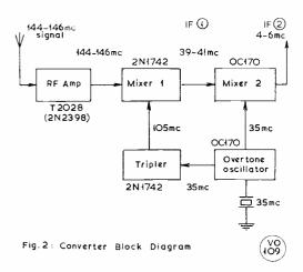
Fig. 2. Block diagram of the G3HRH Converter.
