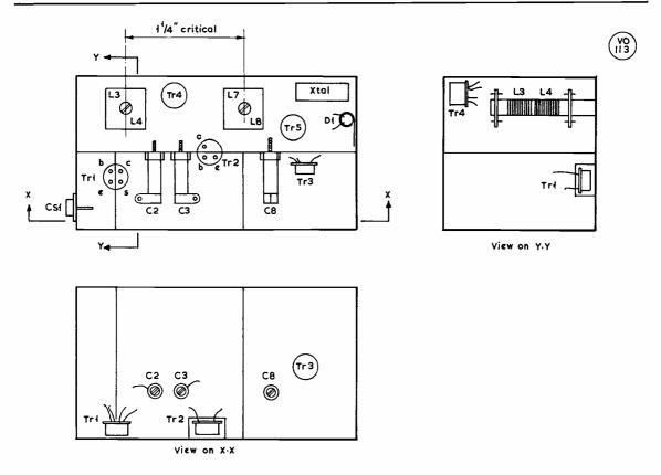
Fig. 6. General layout of components for the Converter.
