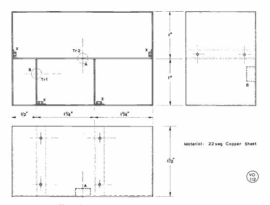
Fig. 5. General arrangement of open-top box with screens.
