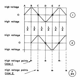
Voltage and current antinodes (points of maxima) on a Lecher line system, maximum current appearing at points O. A half-wave could be measured, physically in centimetres, between points B-D, or D-F, or C-E.
