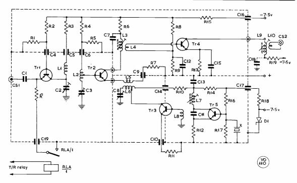
Fig. 3. Main circuit diagram for the G3HRH Converter.
