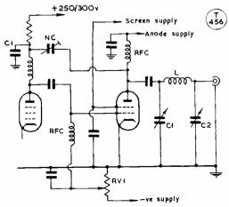
Fig. 2: Typical Class-AB1 Linear Amplifier
