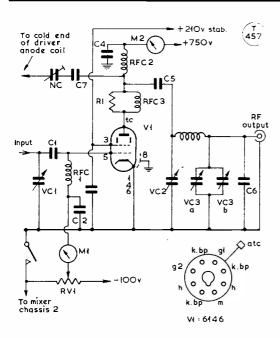
Fig. 3. Typical Class-AB1 linear amplifier, using a 6146, for the 80-metre band. For working on several bands, the pi-tank could be switched. C6 should be in circuit for 80m. and switched out for the higher frequency bands.
