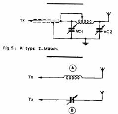
Fig.6: Simple means of loading for one or two aerials
