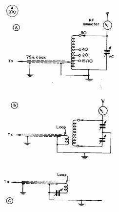
Fig.3 : Tuner circuits to feed 2 gerials
