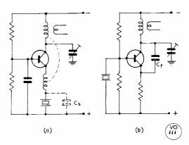
Fig. 4. Alternative overtone crystal oscillator circuits. In (A) Cs represents stray holder capacities. In (B), Cf is a feedback condenser, of about 2.7  $\mu\mu$ F.
