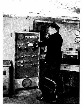
Part of the radio-room of the new Shell tanker "Drupa," showing the main Tx, a Redifon G.341, being set up by the radio officer on one of the many channels and several modes this transmitter provides. To the immediate right of the R/O, on the operating table, can be seen the matching Redifon R.408 receiver.
