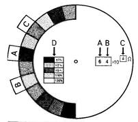
For easy reference just set the colours and the correct resistance value appears in the "window." Also shows resistor tolerance.
