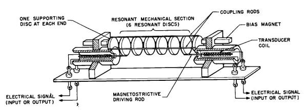
Fig. 8. The physical arrangement of a Collins mechanical filter.
