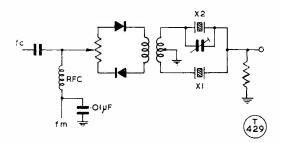
Fig. 14. Method of connecting a half-lattice HF filter to a two-diode balanced modulator.
