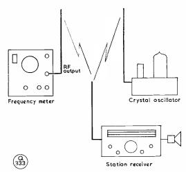
Fig. 5. The station receiver can also be brought in to check on crystal frequency and activity, but an accurate frequency meter is essential for final frequency determination.
