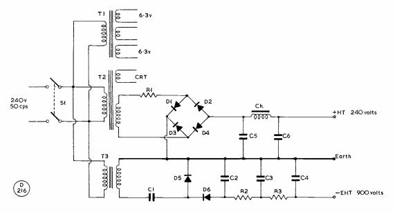
Fig. 11. Power supply section for the Oscilloscope. Values are: C1, C2, C3, C4 0.1  $\mu$ F, 1500v. wkng.; C5, C6 40  $\mu$ F, 350v.; R1 8 ohms 2w. wire-wound; R2 47,000 ohms  $\frac{1}{2}$ w.; R3 100,000 ohms  $\frac{1}{2}$ w.; T1 6.3v. 3A, three times; T2 200v. 200 mA, 4v. 1A.; T3 500v. 5 mA; Ch 5Hy, 250 mA LFC; D1, D2, D3, D4 BY100 or similar for voltage-doubler circuit; D5, D6 J50 or similar rated 500v. at 5 mA.
