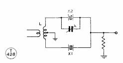
Fig. 13. A half-lattice HF crystal filter. X2 should be about 1.7 kc higher in frequency than X1. Coil L is wound on a ferrite ring as described in the text — and see Fig. 12.
