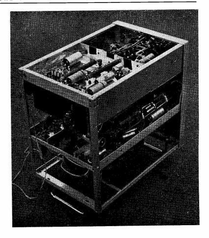
Inverted half-rear view of the Amateur Oscilloscope designed and described by G3OCB. This shot shows the general arrangement of the X-chassis, the power supply section and the rear of the Y-chassis. The tube is in the lower compartment. Note that the assembly is in unit form.
