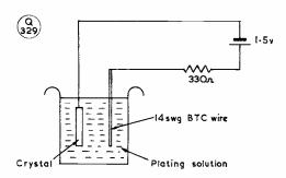
Fig. 1. Circuit used for plating the crystal — see text. The materials should be carefully handled, and it is also necessary to keep a close check on how the frequency change is progressing.
