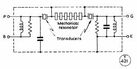
Fig. 5. Diagram to show the general arrangement of the Kokusai range of mechanical filters.
