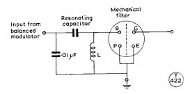
Fig. 6. Showing how a Kokusai mechanical filter can be used to follow a shunt-fed balanced modulator.
