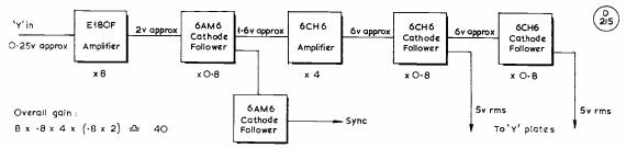
BLOCK SCHEMATIC DIAGRAM OF 'Y' AMPLIFIER
