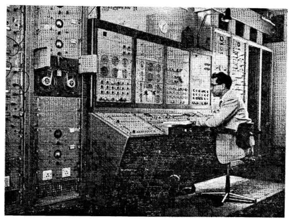
The control room for the new one-mile radio telescope at the Mullard Radio Astronomy Observatory, Cambridge. The dials on the console show the positions of the three telescopes (see text), which are automatically controlled by programme-tape, with read-out, the equipment on the left. The receivers, which are of a very refined high-gain low-noise type, are grouped in racks on each side of the operating console.
