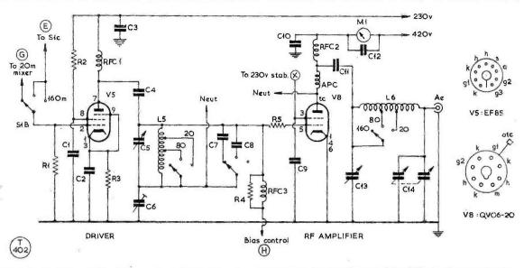
Fig. 3. In the Sphinx Sideband transmitter for 20-80-160 metres, the driver (V5) is an EF85, and the PA a QV06-20 with neutralisation, the screen voltage being stabilised. A great deal of design work has gone into the achieving of a stable unit capable of developing its full RF power output of about 70 watts p.e.p.
