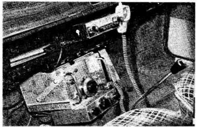
Seen at the Worcester Club's meeting at Callow End: The G3SMT/M installation for 160m. fitted in his MG-1100. The rig is a 10-watt Tx with a 160-metre converter feeding the car receiver as IF/AF amplifier.
