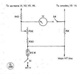
Fig. 1. The S-meter circuitry in a standard HRO receiver, which is worth modifying for the reasons explained in the article. The necessary circuit changes are shown in Fig. 2.
