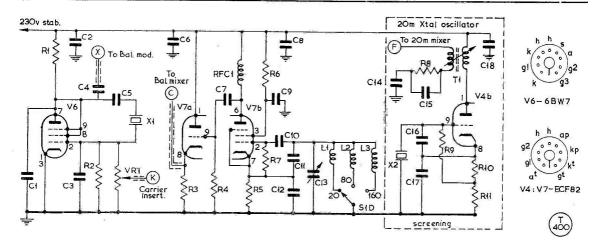
Fig. 1. Circuit arrangement for the originating stages in the Sphinx Sideband transmitter, showing the carrier oscillator V6 (a 6BW7), the VFO and cathode follower V7 (ECF82), and the crystal oscillator for 20 metres, the triode section of an ECF82.
