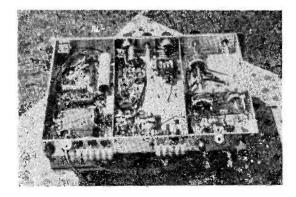
An impression of the interior construction of the Sphinx. Good-quality components, proper screening, and sound design both mechanically and electrically contribute to stable, high quality output.
