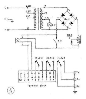
Fig. 4. The Delta Control unit used with the Sphinx SSB Tx, to give press-to-talk operation. As explained in the text, this is the sort of control circuit that could be used with any transmitter—it is just a matter of connecting the relay circuitry to give the c/o motions required.
