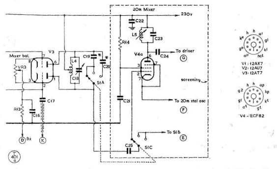
Fig. 2. This circuit, which should be read from V1 at the left-hand edge of the opposite page, shows the audio, balanced modulator, Sideband filter and 20-metre mixer stages. As indicated, certain component values are selected for each individual unit—most other values of interest are given in the table opposite. The lettered points are for inter-connection into other parts of the circuit as a whole.
