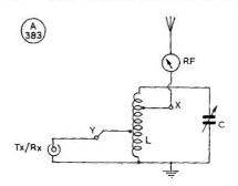
A simple aerial tuning unit for use with a random-length wire fed against ground. Adjustment is discussed in the text and, for multi-band operation, the coil may be tapped and switched as at X and Y, using a third wafer on a ganged ceramic switch. The construction of the coil should be such as to give the best possible Q-factor. The RF meter, which can be an 0-500 mA or 0-1 amp. thermo-couple instrument, will be found very useful for adjustment.
