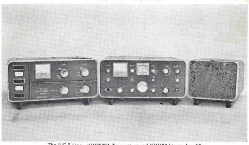
The "G" Line-KW2000A Transceiver and KW600 Linear Amplifier.
