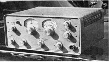
Shown at the Barford Rally — the very fine 20-80-160m. Sideband transceiver built by G3HVX (Hereford). Beautifully constructed, it has a separate dial (left) for the IF incremental tuning control on the Rx side; this enables the receiver to listen off the Tx frequency.
