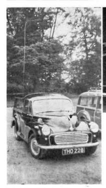
Seen at the R.N.A.R.S. Rally — a Top Band whip of somewhat inordinate length. The loading coil is about half-way up the aerial
