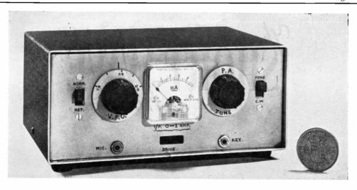
How the miniature mobile Tx, as designed and constructed by G3SRY, looks when completed — note the half-crown for size comparison. The PA consists of a pair of Mullard AUY10's, running the full 10 watts input on 160m. from a 24-volt supply line, loading to just over 400 mA. The design incorporates VFO control, and high-level modulation is by another pair of AUY10's — see circuitry.
