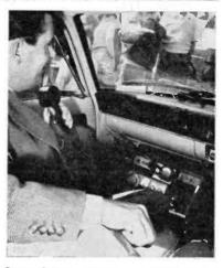
Seen at Saundersfoot, June 20. GW3MOP/M has his 160m. gear in a neat wooden case; the rig consists of a Command Rx and Codar A.T.5 Tx, easily removable for /P or fixed-station use.
