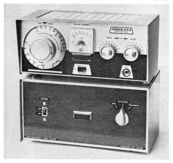
The AT5 transmitter and the Type 250/S power supply are similar in size, and, standing as shown, take up an area of only 8½in. by 5½in. The three-position switch at the right of the PSU gives complete switching of both transmitter and aerial. The neon indicator in the centre of the PSU shows a steady glow on "net" and "transmit," and flashes intermittently on "stand-by"; that in the centre of the transmitter's front panel gives indication of modulation.
