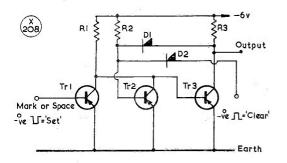
Fig. 5. To obtain "mark" and "space" latches — see text. Resistors R1, R2, R3 are each 1K; D1, D2 can be any germanium diode; and the transistors are of the type MAS21, MA393, or MDS33.
