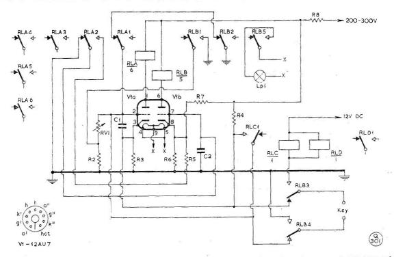
Circuit of the control system for "send-receive," devised by EI5AN for the protection of a receiver having a transistorised front-end. Matters are so arranged that the Rx is cut right off before the transmitter can radiate any RF, nor can the receiver come on until after radiation ceases. The whole change-over operation is controlled by the key, with a slight time-delay to hold the transmitter "on" during a keying session at normal speed — all explained in the article.
