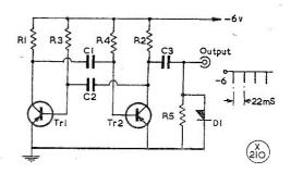
Fig. 7. A timing multivibrator, in which Tr1, Tr2 can be any low power transistor; D1, germanium diode; C1, C2, 3.3  $\mu$ F for a 22-millisecond period, possibly requiring trimming; C3, 1  $\mu$ F; R1, R2, 470 ohms; R3, R4, A-7K, adjustable for final timing; and R5, 1K.
