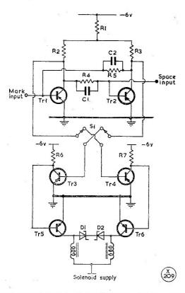
Fig. 6. Output stages for the RTTY receiver. The transistors Tr1, Tr2, Tr3, Tr4 are as in Fig. 5, with OC36's or any equivalent for Tr5, Tr6. Other values are: C1, C2, 470  $\mu\mu$ F; R1, R2, R3, 470 ohms; R4, R5, 47K; R6, R7, 330 ohms. For D1, D2 see text.
