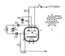
Circuit of the magic-eye GDO. Values for L are given in the table. C1 is  $100 + 100 \ \mu\mu$ F connected series-gap; C2, C3 are 82  $\ \mu\mu$ F; C4 is .002  $\ \mu$ F; R1, R2 are 1 megohm each; R3 is 22,000 ohms; and the valve is an EM84, which has the deflector connection brought out separately.
