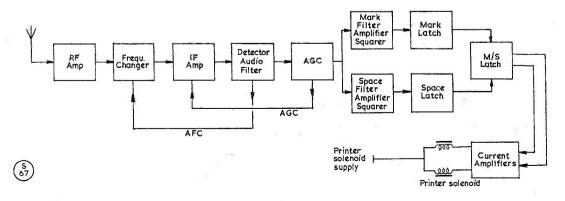
Fig. 4. Block diagram for an RTTY receiver, using some of the circuits discussed in the text. The characteristics of transistors lend themselves admirably to any circuit situation where switching, at any speed, is involved.
