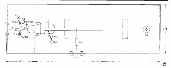
Fig. 2. This sketch is to almost exactly half-size, and shows the mechanical layout of the circuit of Fig. 1. The valve is a disc-seal triode, type DET-22, in which the grid connection is made to a copper ring, this forming the earthing point when the valve is mounted in the screening panel. The depth of the trough is two inches, and other details are given in the text.
