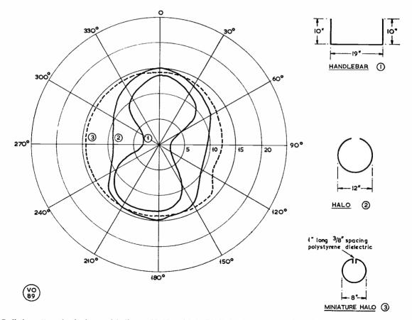
Radiation patterns for the three aerials discussed in his article by G4AC, showing the halo configuration appropriate to each pattern. These are for the two-metre halo's, at a frequency of 144.2 mc, with an SWR of 1.1:1 exhibited. The gamma matching feeds are 4in. long with a 4.7  $\mu\mu$ F series condenser. G4AC claims much improved performance when using these shapes under mobile conditions.
