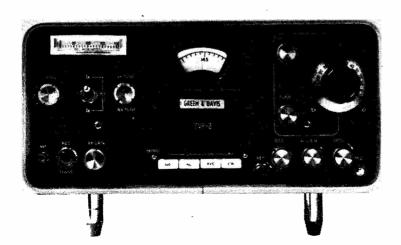
The Green & Davis TVR-2 is a transistorised 160/2m. transceiver, featuring modular construction, the only valve used being a 7558 for the PA—this could be replaced by a suitable transistorised PA when it becomes available. In all, 28 semi-conductors are involved for Rx and Tx, construction is on printed circuit boards, and each module is separately screened, with the oscillator and mixer stages in die-cast boxes.
