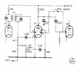
Fig. 2A. The original circuitry involving the detector and AVC line in the Hig-30. Some suggested modifications are shown in Fig. 2B. It should be noted that the circuit designations are in accordance with the manufacturer's handbook on the receiver.
