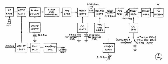
Fig. 1. Block diagram of the all-band Sideband Exciter described in the article by G3OCB. While it could be operated initially as a low-power S3B transmitter — the PA vive being a 5B/254M — it is intended as a driver for a 600-watt linear amplifier. On the constructional side, the arrangement breaks down into five separate units, made up as sub-assemblies for mounting on a single chassis. Details of the circuitry are shown in Figs. 2-4 herewith.
