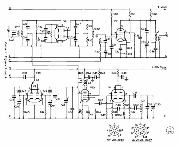
Fig. 3. Circuitry for the VFO and Sideband selection in the G3OCB SSB Exciter. The latter operation is performed by S2, in the plate of V3, and values for the appropriate crystals are given in the table. V11 is the VFO, and V10 its amplifier stage, since the output from V11 is kept very low in the interests of stability. Further details are given in the text, and it will be noted from the lettering how Fig. 2 connects to the next section and how Fig. 3 feeds into Fig. 4.
