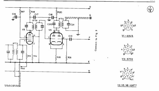
Fig. 2. The audio, carrier and filter section in the Sideband Exciter by G3OCB. This is fully discussed in the text, and the crystal frequencies to use are given in the table on p. 660. With full filtering, a very high degree of carrier suppression can be obtained.
