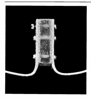
Close-up of the solid-dielectric capacity loading section, actual size, on an 8-inch diameter Mini-Halo for two metres, as designed by GAAC.
