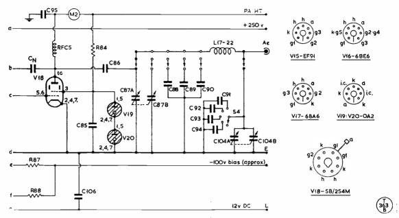
Fig. 4. The final conversion, driver and RF power amplifier section of the Exciter. The output at V18 is for all bands 10-80 metres, the small capacities C37 and C104 being selected and loaded as required for the correct L/C ratio from band to band. This is partly achieved by the way the plug-in coil mount is wired for the different bands. This section of the circuit connects into Fig. 3 as shown by the side lettering.
