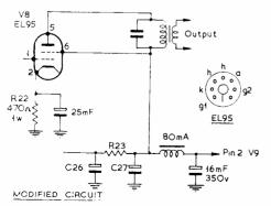
Fig. 1. The original output end of the HE-30, as modified by G3GDJ and explained in the text.
