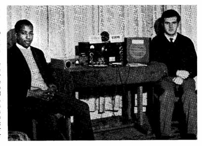
The Grafton Radio Society, signing G3AFT, came out a very creditable fifth, with 564 points, in the 1964 MCC — a position much improved over theirs of recent years. The gear consisted of an HRO-5T, and the Tx was a 3-stage job using a 5B/254M in the PA; the aerial is described as "a 3/4-wave Marconi, with a 50ft. vertical section, and buried radials"—it certainly put out a very potent signal. Operators on G3AFT were Neville Bethune (G3RFS), left; and Keith Spicer (G3RPB).
