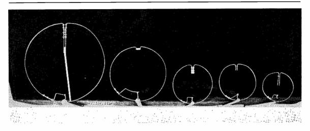
Mini-Halo aerials for mobile, as evolved by G4AC, ranging from 6 inches to 12 inches in diameter for two metres, and 18 inches for four metres. These aerials were designed and constructed for the tests discussed in his article.
