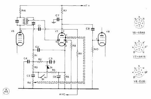
Fig. 2B. This is the circuit of Fig. 2A, as modified in accordance with the details given in the text. The switch Sw controls the new noise-limiter circuit, taking the diode D1, an OA70. The first IF transformer is T4, as in Fig. 2A, and R16 is as in the original. These fairly extensive modifications, for which all values are given in the table, are claimed by G3GDJ to improve the HE-30 considerably.
