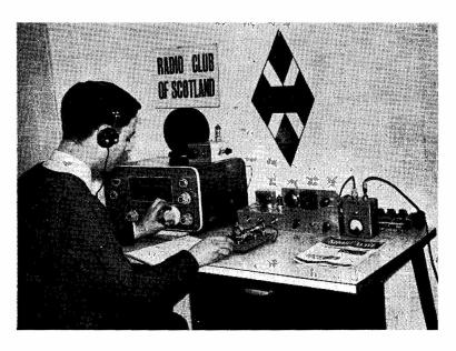
Neat Top Band rig at GM3RCS, of the Radio Club of Scotland. The station was specially assembled for the 1964 MCC; the operators were GM3LTB, GM3SAN (seen here) and GM3SJU. Their Tx was to a "Short Wave Magazine" design, using a 6BW6 in the PA, and full BK with a valve-type T/R switch. The receiver was a Minimitter MR44/II, and the aerial an inverted-vee with a maximum height of 38 feet. In 16th place, and leading the Scottish entry, GM3RCS made 492 points.
