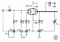
Fig. 1. Circuit of the 70-centimetre pre-amp. described by G3NDC, using a DET-22 in grounded grid. A physical layout for the trough, with dimensions, will be found in Fig. 2.
