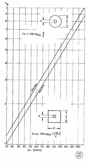
Fig. 1. Ratio of inner conductor diameter to outer conductor dimension, D/d, plottled against impedance, Zo, for both square and circular outer conductor.
