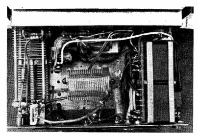
Upper chassis view of the 30w. transistor Tx, showing the PA tank assembly; the coil, L3 in the diagram, has been made high-Q and its constructional detail is given in the Table of Coil Values. In this picture, the modulation transformer T3 is to the right, and the mounting for the four meters (out of their cases) is visible along the top of the photograph. The 2N1046's in the PA are mounted with cooling fins.
