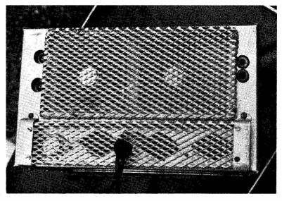
Rear view of the E17A 80m. TTx, running a good 30 watts, fully modulated, using transistors only. Since those mounted on the rear panel dissipate some heat, speaker grille material is fitted to provide ventilation.
