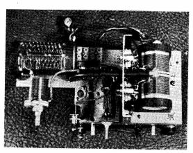
Showing stages in the construction of the G3AM TTx. Below is the ATU/PA section with the tapped aerial tuning coll L9 and its tuning condenser C20, on the left. The PA transistors can be seen grouped on the vertical panel, looking into the L7, L8 assembly.
