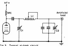
Fig.3. Typical pi-tank circuit
