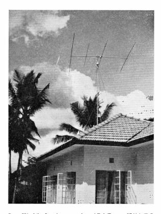
On p. 229 of the June issue, we showed Bob Tanner, 5Z4AA (P.O. Box 5121, Docks, Mombasa, Kenya) in his station. Here is how the QTH looks from outside, with the Hygain TH4 for 10-15-20m. at a height of 47 ft. This beam is controlled by an AR-22 rotator, and is fed through 52-ohm balun matching.
