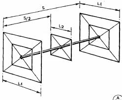
Fig. 2. Composite 2metre/4metre array
