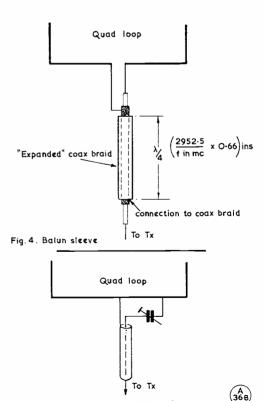
Fig. 5. Two metre gamma match section
