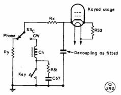
Fig. 6. Keying circuit for the G3RKK transmitter, when breaking V5 cathode: C67, 1.5  $\mu$ F; R51, 100 ohms; R52, 220K 1-w.; Ry = DC resistance Ch.; Rx + Ry = Cathode res. as originally fitted; Ch., 2 Hy 100 mA. If keying at V4: C67 is 1.0  $\mu$ F and Ch. is 5 Hy 20 mA. See circuits Part 1 June issue for references.
