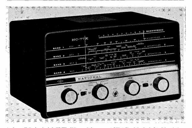
Another new National receiver is the NC-77X, which covers the frequency-range 540 kc to 31 mc in four bands. Intended as a beginner or SWL receiver, it is in the lower-priced category, but has separate electrical bandspread and a built-in speaker. It is very nicely finished, in a grey-blue steel cabinet with brushed aluminium front panel.
