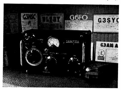
The completed G3AM TTx described in the article. It has now been in use on 80m. for more than three months. In that time all the U.K. has been covered, also Northern Europe as far as UA1. The cards in view confirm some of these contacts, obtained with a PA input of about 750 milliwatts only. An essential factor for success is a good ATU, as shown in the main circuit diagram, and a reasonable aerial. Though the VFO is fundamental, the buffer amplifiers ensure stability and a good T9 note.
