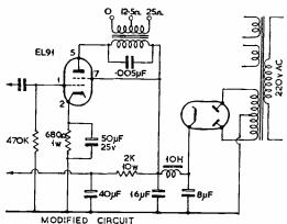
These circuits explain the modifications suggested in the text. The Lafayette HE-30 is a good general-coverage receiver which can be improved on the audio side by these simple circuit changes.
