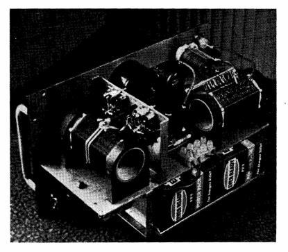
General view, half-rear, of the construction of the G3AM transistorised 80m. CW transmitter. As explained in the text, it built in units, these forming the necessary screening partitions, since all five stages are on the same frequency. The PA tuning coil L7 is at left, with the link L8 for coupling into the ATU coil L9 — see text and Fig. 1.
