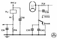
Fig. 7. When the G3RKK Tx is used mobile or portable, the PA clamping circuit can be by relay, as shown here and originally described by G3LWM in the December 1963 issue of "Short Wave Magazine." Condensers C31, C32, C33, C39, C40 and R16, R21 are as fitted in Fig. 3 on p.221, June 64. In the circuit above, R1 is 18K, to equal the DC resistance of Ry (R1 and Ry replace R15) and Ry is any relay with a 2 mA coil, having contacts rated at the control voltages involved.
