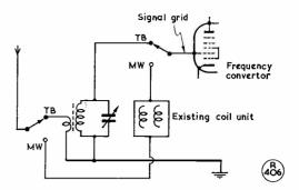
Circuit arrangement to obtain signal input at the image frequency, applicable to any MW/BC Rx for Top Band reception.
