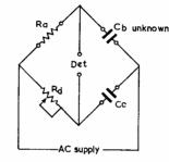
Fig. 4. Capacitor Testing
