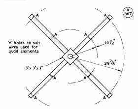
Fig. 3a. Support 'spider' for large end section
