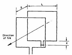
Fig.1. Basic two element quad.
